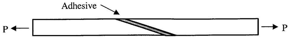
Figure 2-1: Diagram of a scarf joint
