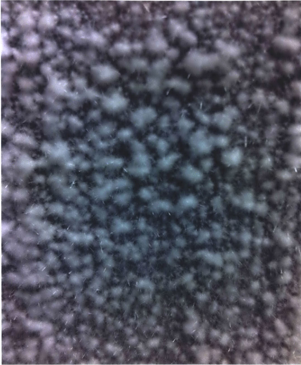
Figure A.8: Gypsum Scale Layer at T=50^{\circ}\text{C} and SI=2.4
