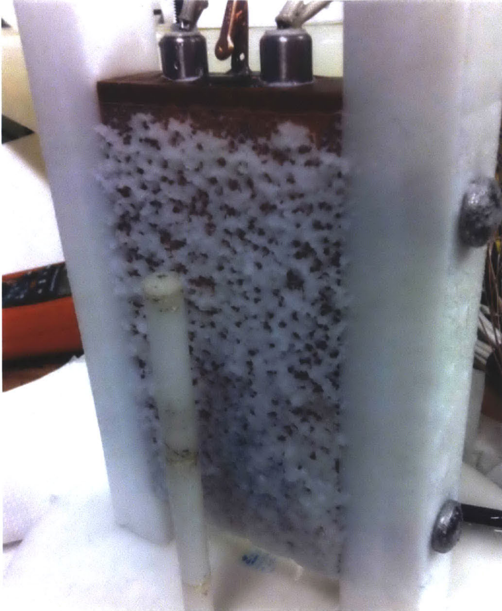
Figure A.7: Gypsum Scale Layer at T=40^{\circ}\text{C} and SI=2.4
