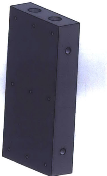
Figure 2.4: Locations of Monitoring Thermocouples
