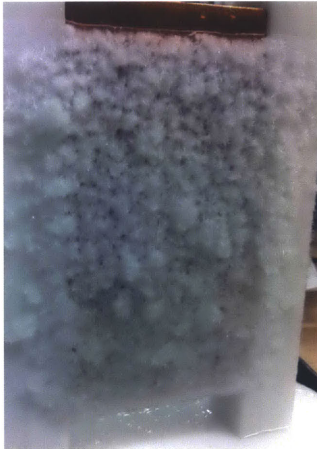
Figure B.2: Gypsum Scale Layer at T=80^{\circ}\text{C} and SI=4.0 without EDTA
