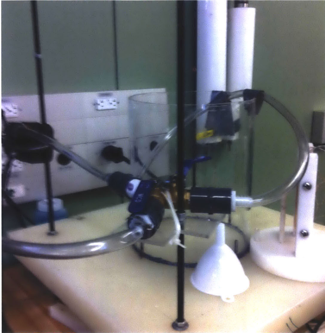
Figure A.2: Recirculation Pump Component System
