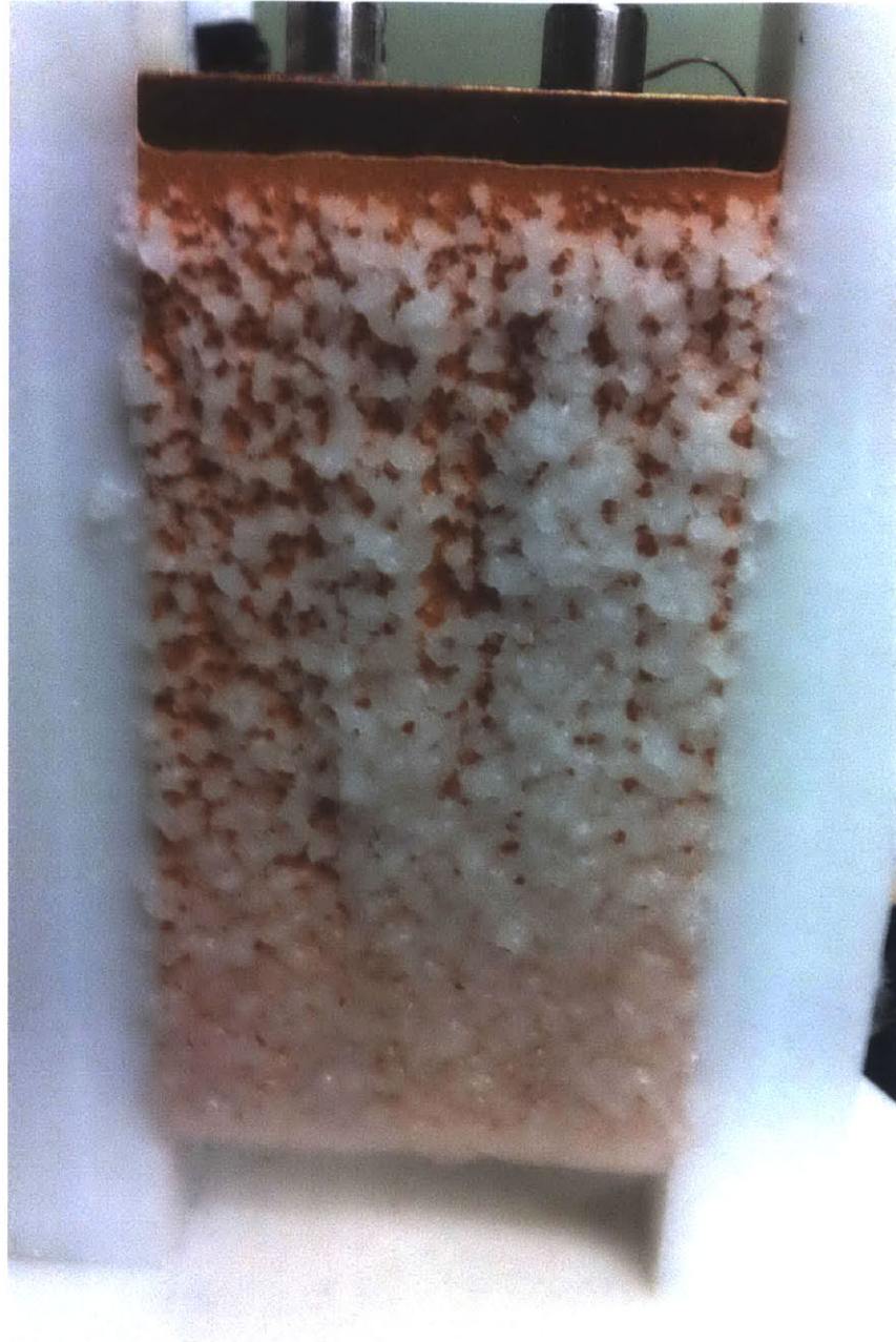
Figure A.9: Gypsum Scale Layer at T=60^{\circ}\text{C} and SI=2.0
