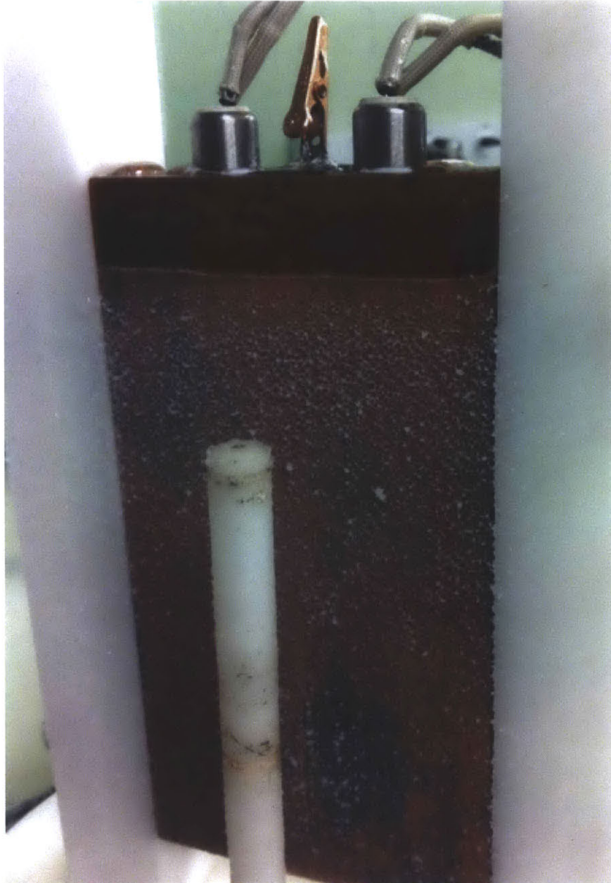
Figure A.5: Gypsum Inception Layer at T=80^{\circ}\text{C}
