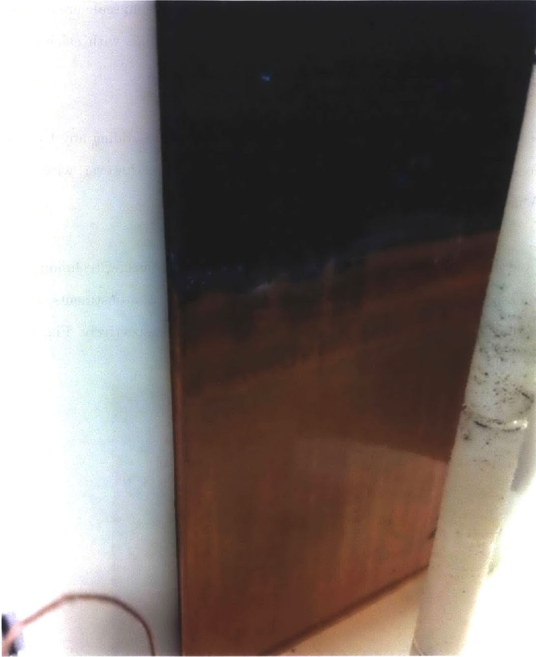
Figure B.3: Gypsum Scale Layer at T=80^{\circ}\text{C} and SI=4.0 with EDTA
