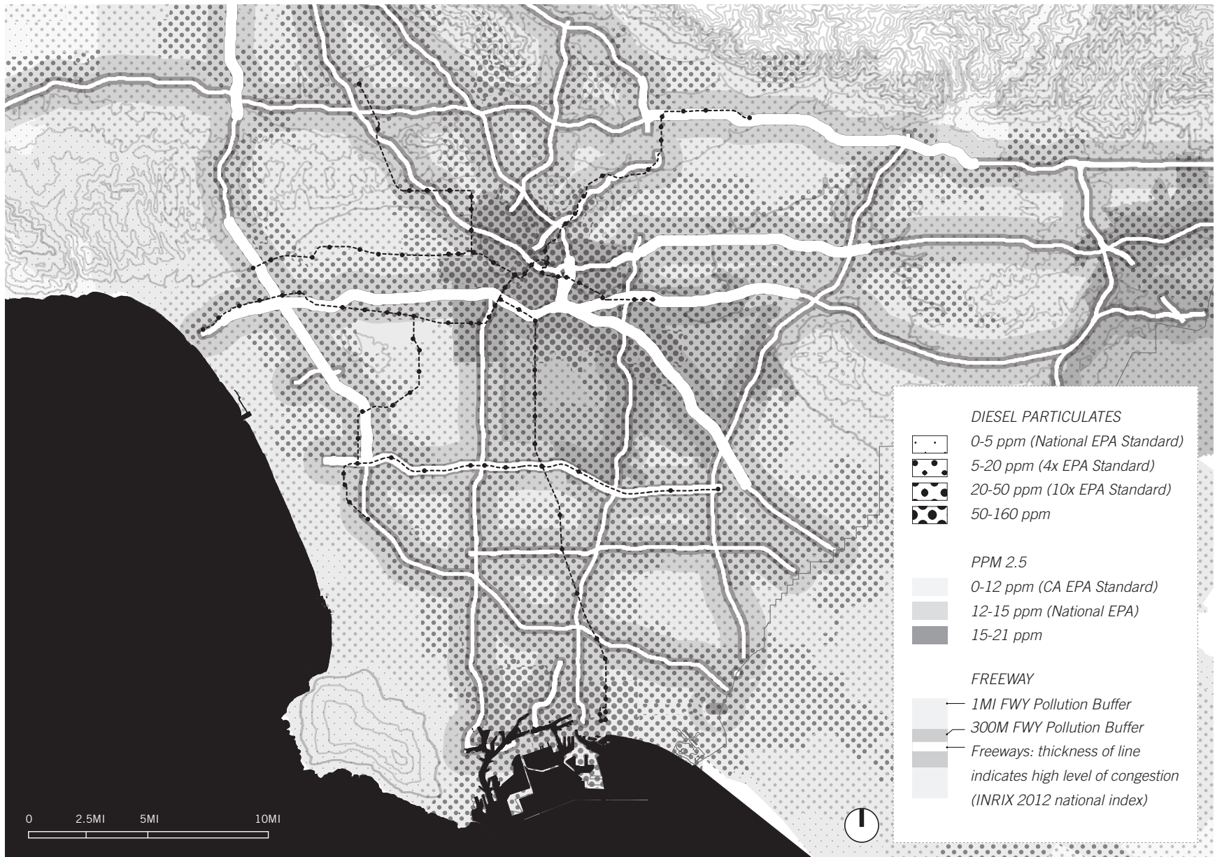
Diesel Particulate Matter (DPM) & PPM 2.5 (Ultra Fine Particulate Matter), (California EPA / CalEnviro Screen Website, 2013)
