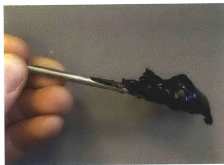
Figure 1-4: Image of a typical waxy crude oil below its wax appearance temperature T_{wa} (sample provided by Chevron). The material clearly holds its shape and does not flow - behavior indicative of a yield stress fluid.
