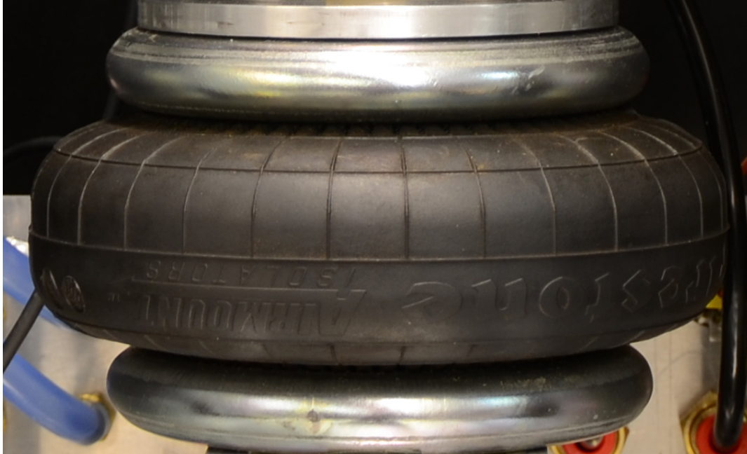
Figure 4-4: Firestone AirStroke Pneumatic Actuator: The actuator consists of a specially shaped and reinforced rubber cylinder between two metal plates, which have fixtures for mounting.
