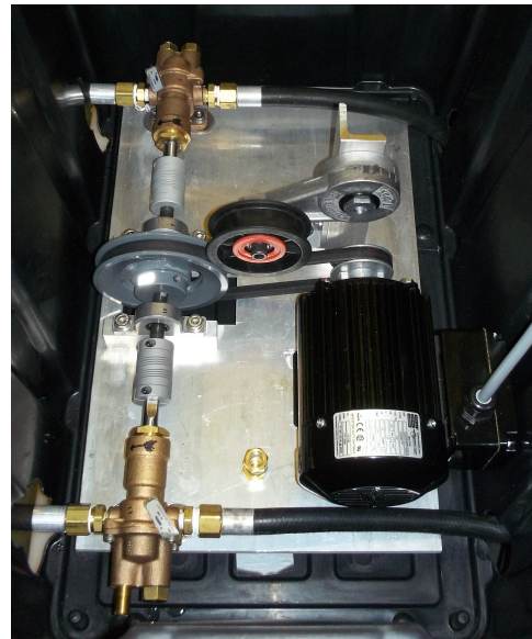
(b) Photo of Gear Pump System
