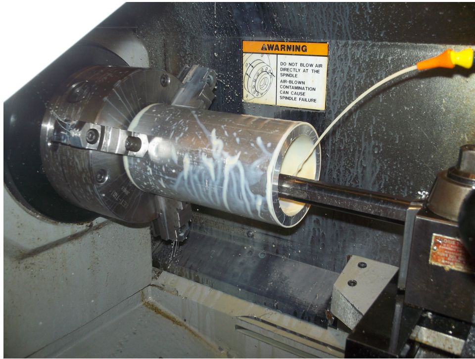
Figure 5-5: Boring ID of Aluminum Housing on HAAS CNC Lathe
