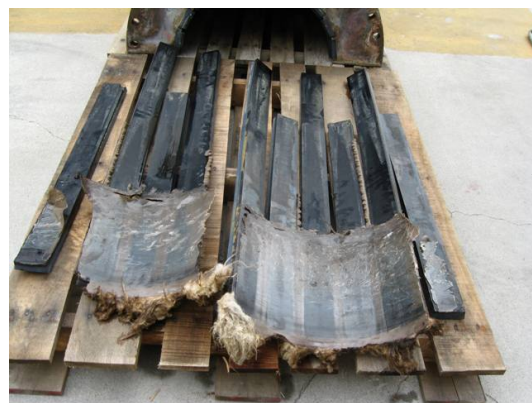
(b) Stave bearing failure due to ingestion of foreign debris
