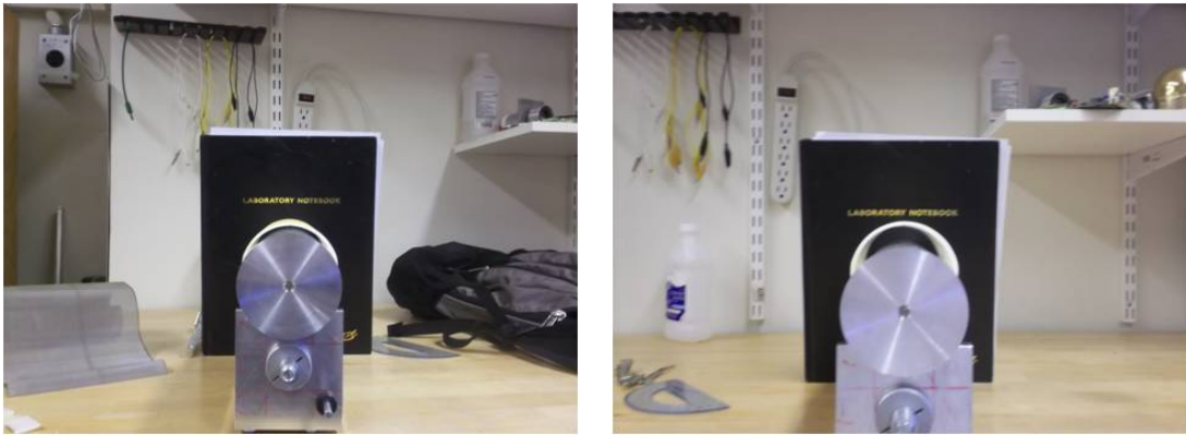
(a) UHMW PE 5 minutes after removal from master shaft (b) UHMW PE 24 hours after removal from master shaft
