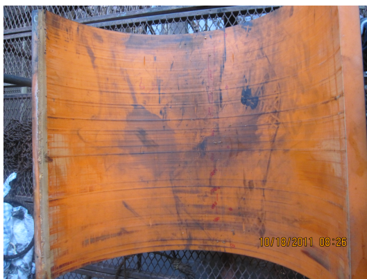
(a) Plain journal bearing failure
