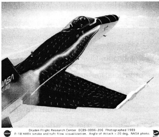
Figure 1-2: Experimental feature identification: F/A-18 leading edge extension vortex visualization using smoke in flight [9]
