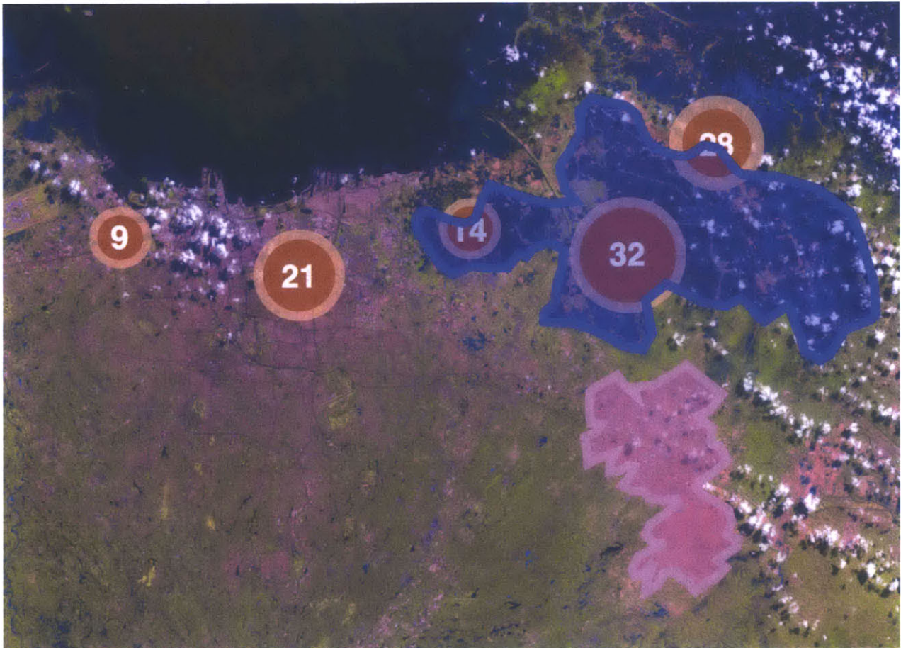
Concept image of IR data combined with participatory data (red circles). IR data can help highlight areas of refuge (pink outline) and vulnerability (blue outline). Combining maps of these areas with participatory data could help planners and responders better allocate resources for citizens during emergencies.
