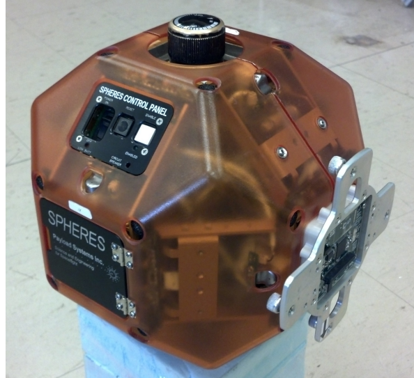
Figure 7-1: SPHERES With Expansion Port
