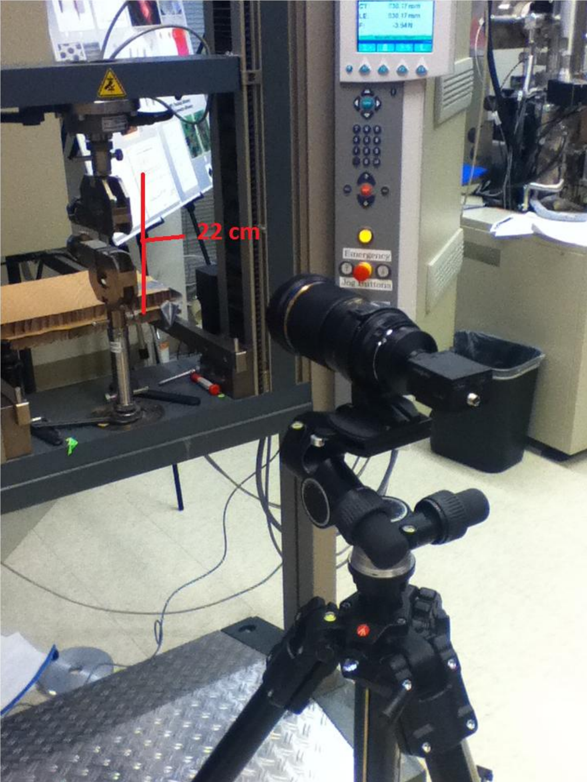
Figure 3.8 MIT 2-D Tensile Testing Setup. Tensile testing machine is on left with camera/tripod on right.
