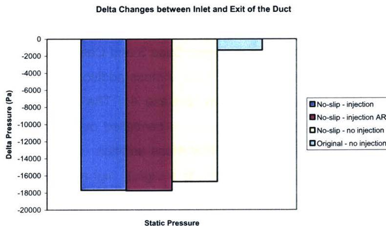
Figure 5.2.20. Pressure changes between inlet and exit of the duct
