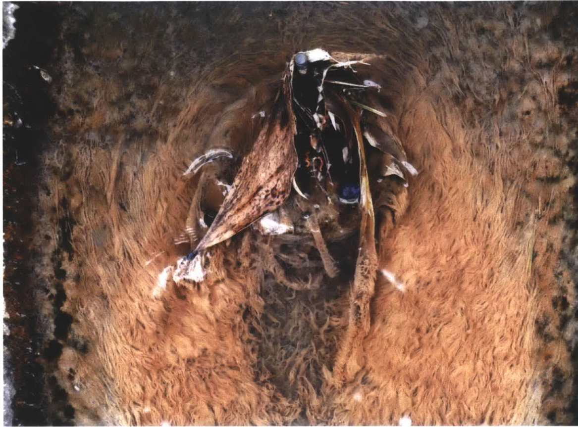
Figure 1. Biofilm growth and accumulated leaves around concrete coupon in a storm drain located in the Verde View neighborhood of Singapore on December 28, 2012 (Ekklesia 2012).
