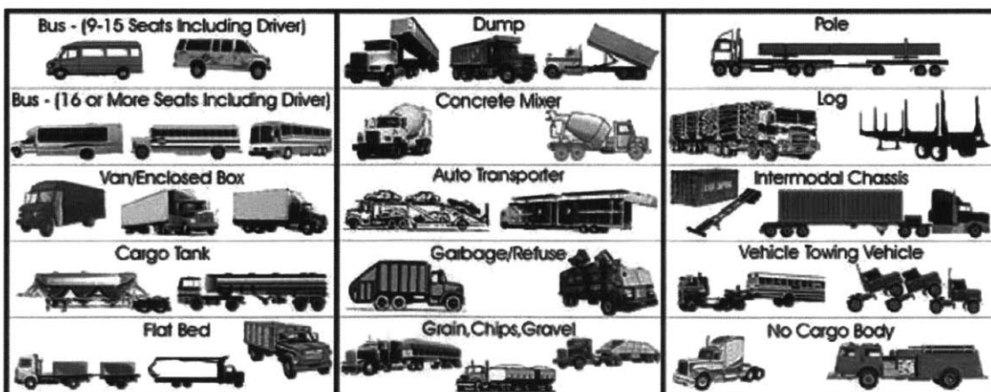
Figure 2-3: Different trailer types (Source: FMCSA 2011a [32])
