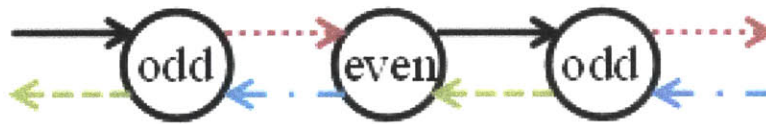
Figure 3-4: Nodes are assigned even and odd numbers so that each link connects one odd and one even node. Nodes sharing a color and pattern can be activated simultaneously.
