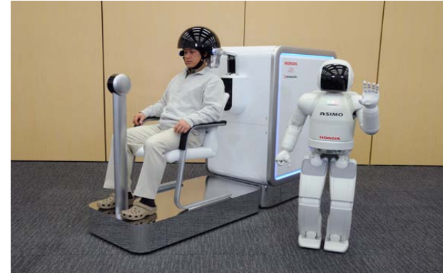
Honda, ATR and Shimadzu Jointly Develop Brain-Machine Interface Technology Enabling Control of a Robot by Human Thought Alone, Honda ASIMO, retrieved from http://world.honda.com/news/2009/c090331Brain-Machine-Interface-Technology/
