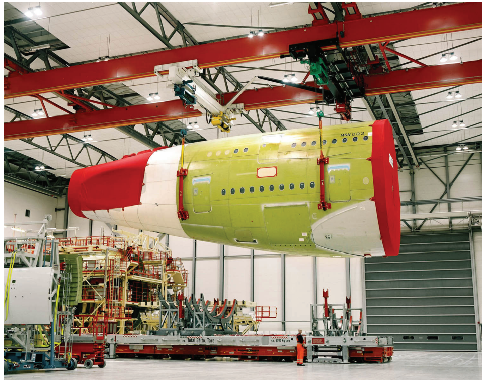
Figure 5-1: A crane transports a part of the Airbus A380 fuselage, in the final assembly line factory in Hamburg, Germany.
