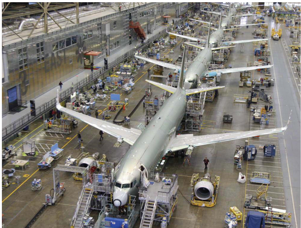
Figure 6-2: Boeing 737's Final Assembly Line (FAL), after the company switched Lean Manufacturing methods.
