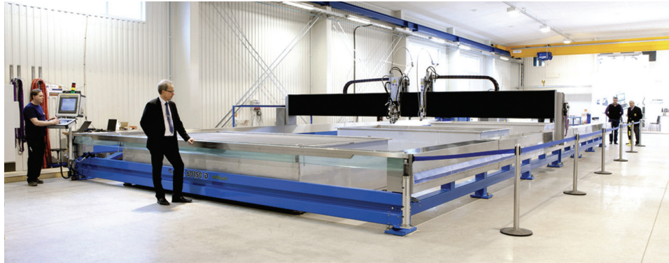
Figure 7-2: Water Jet Sweden AB's water-jets machine with abed size of 6 X 20 meters.
