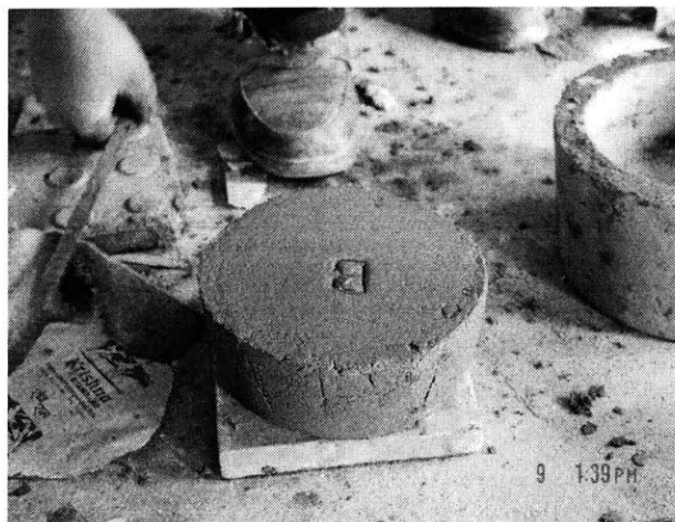
Figure 7-14: The mold is carefully inverted to remove the mixture and is labeled for easy identification.
