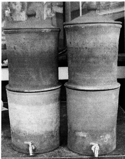
Figure 8-4: Two Thimi ceramic filters with ceramic filter disks of different compositions that are brought back to MIT.
