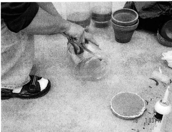
Figure 7-7: Cutting the bottom part of the plastic containers purchased from marketplace.
