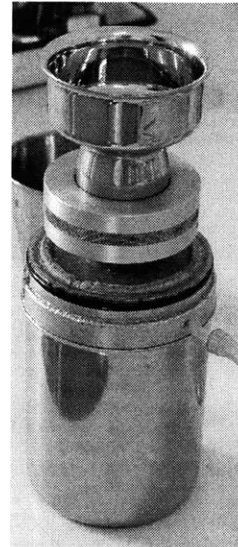
Figure 6-2: Portable Millipore stainless filter holder.
