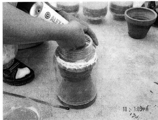
Figure 7-8: Filter disk placed in the plastic containers and silicone applied all around for water sealing.
