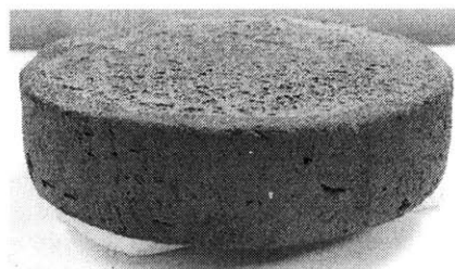
Figure 8-3: TERAFIL ceramic filter disk.
