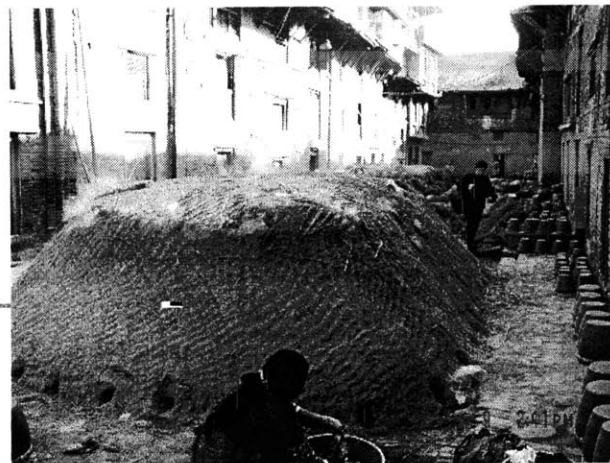
Figure 7-4: Pots are fired between 3-5 days in covered ash mound with small side vents emitting smoke.
