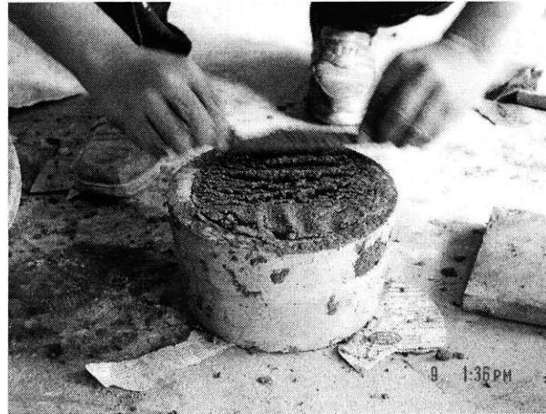
Figure 7-13: Excess is scrapped off to form a smooth surface after pressing and filling the mixture to the top.
