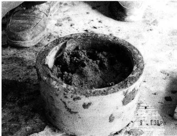
Figure 7-12: Mixture placed in a plaster mold made by Hari. The mold has an inner diameter of 6" and depth of 3".
