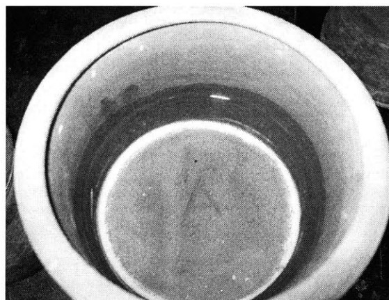
Figure 8-5: Top view of the upper container showing the ceramic filter disk A.
