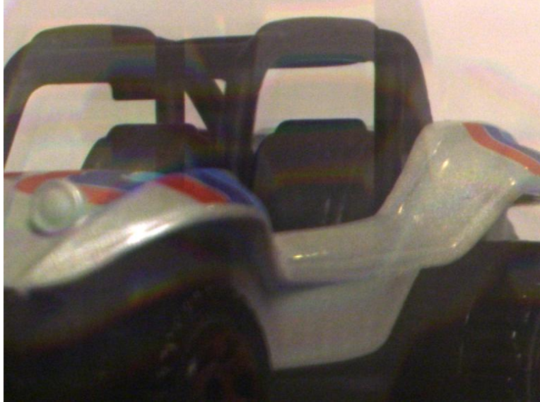
Figure 3-5: An image from one of our early light fields. The picture exhibits heavy ghosting, a result of the LCD behaving as a 2D diffraction grating. The ghosting effect is particularly noticeable around the Matchbox car's front fender.
