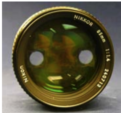
Figure 1-2: Two off-center apertures on a single aperture plate
