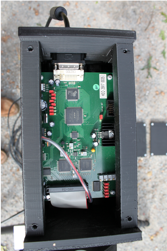
(c) Holoeye HED-0017 driver board. The apparent warping of the parts is actually radial distortion from the wide-angle lens that capture the photo.
