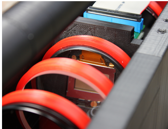
(d) Close-up of the Sony microdisplay as seen through the 2nd & 3rd lenses
