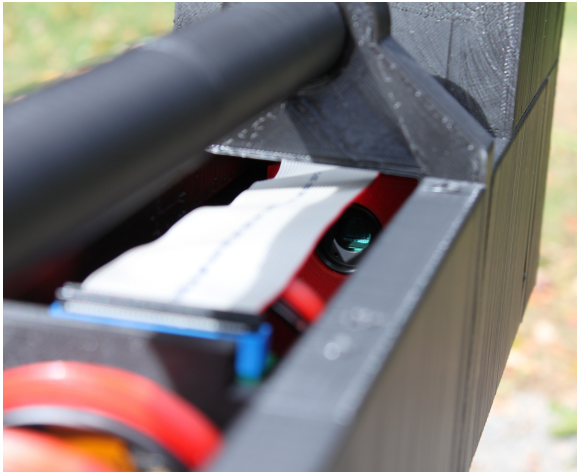
(a) AVT Stingray sensor at rear of optical cavity, barely visible under the ribbon cable that connects the microdisplay to the driver board
