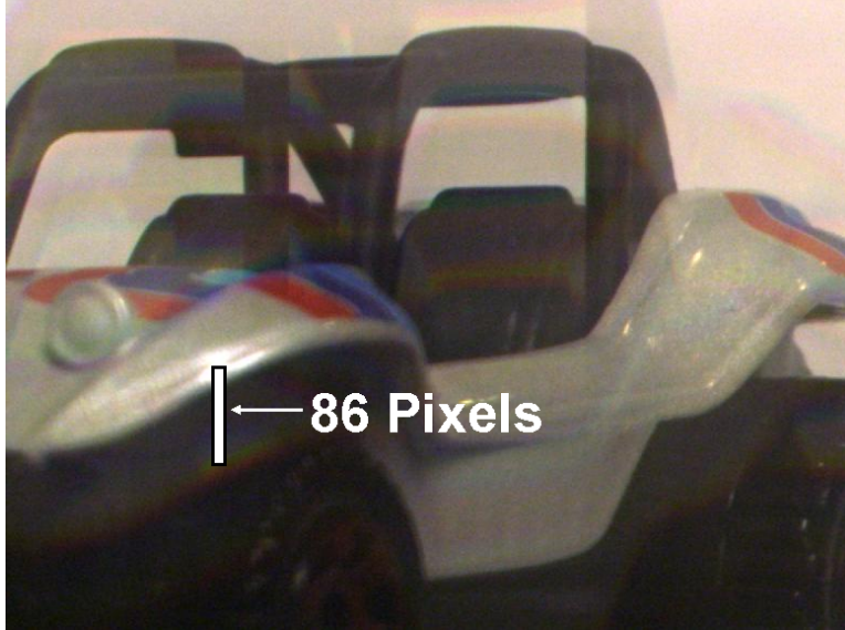
Figure 3-8: This is the same image as in Figure 3-5 with the vertical 1st-order ghosting distance measured in white.
