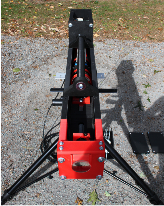
(a) 4th-generation camera with lids removed to reveal the optical cavity
