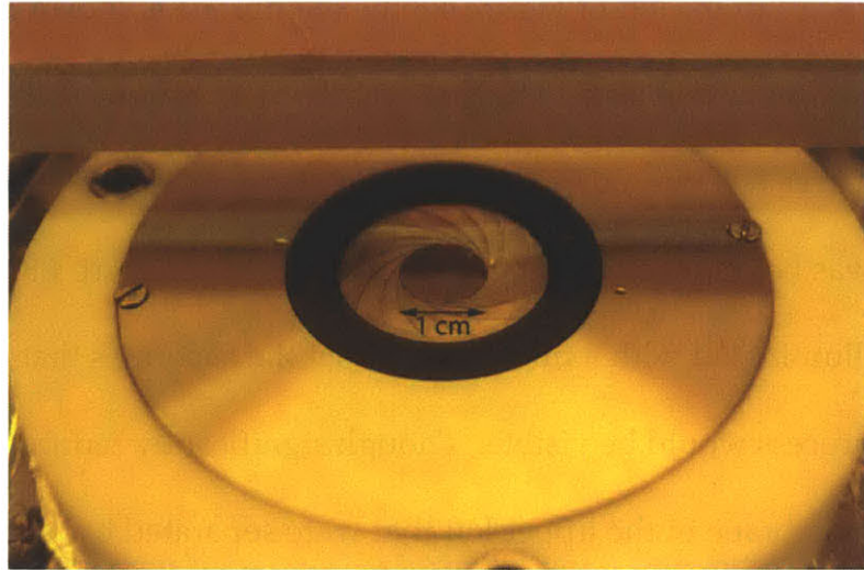
Figure 4.6 Iris-based membrane stacking apparatus. (a) Blown up design of second membrane stacking apparatus illustrating the base, adapter and adjustable iris. Water supplied from the right could be drained from the left. Tip/tilt screw were included to level the apparatus. Though depicted in (a) the air tube was not used. (b) The 1-cm-diameter membrane is shown floating inside the aperture of the iris.
