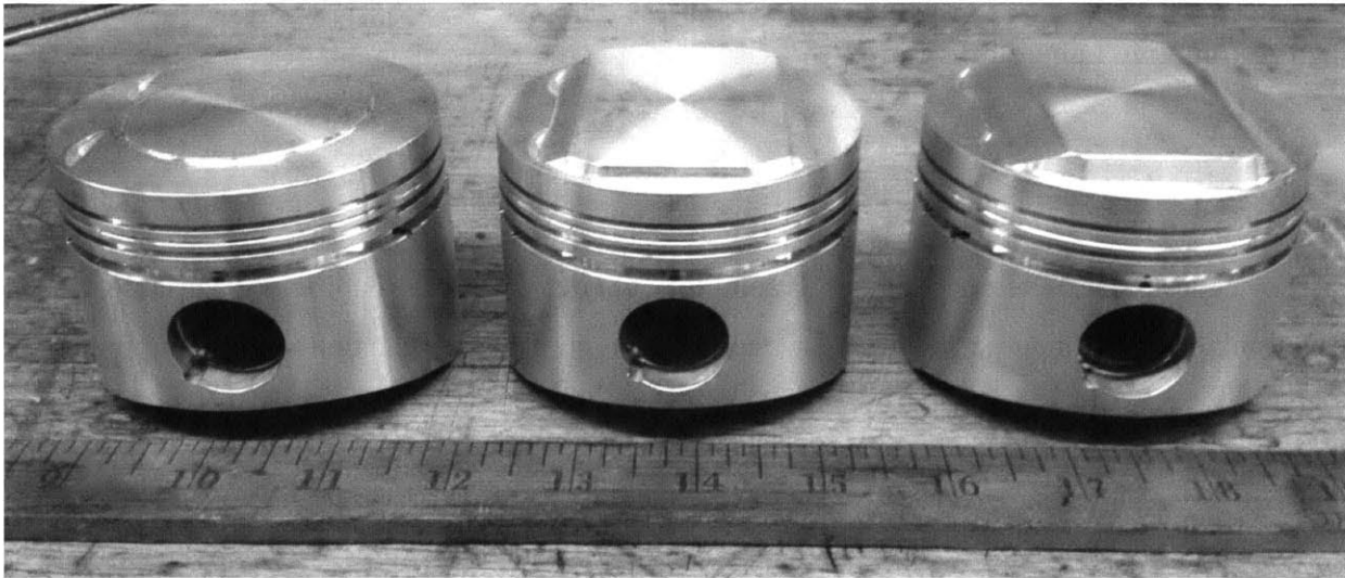
Figure 3-1 Low, medium, and high compression ratio pistons, left to right.
