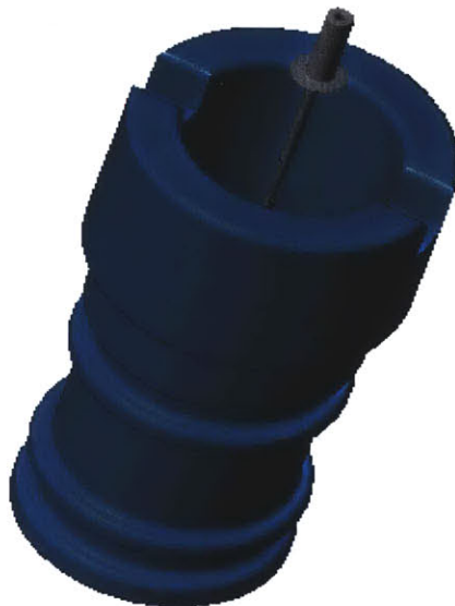
Figure 7-4: Blind Assembly of Main Poppet and Main Poppet Retainer
