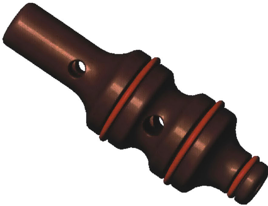
Figure 8-2: Side Poppet Sub-Assembly Redesign
