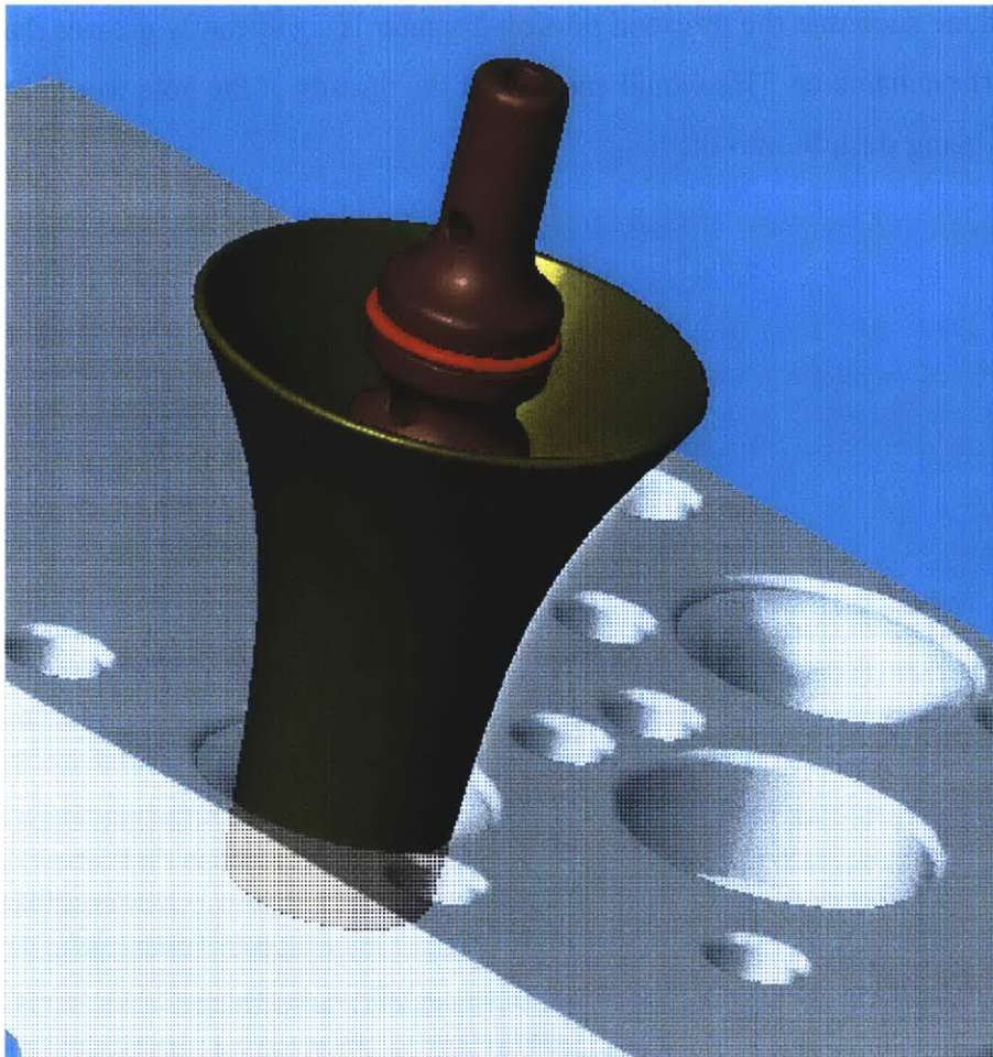
Figure 8-6: Stuffer Insertion Technique
