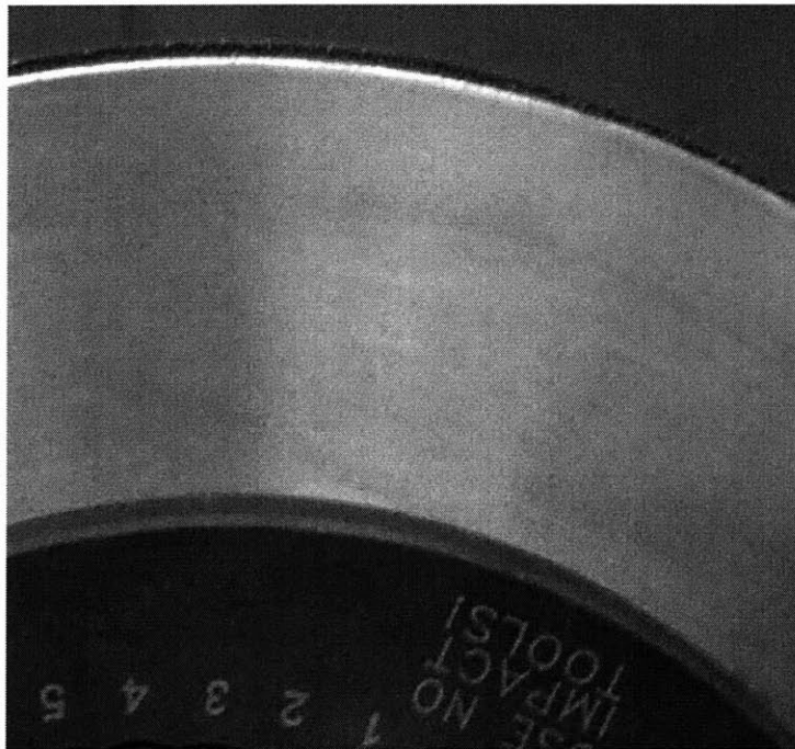
Figure 5-9: Prototype 2: output 50 \mu -inch surface finish at 0.010" depth of cut per side
