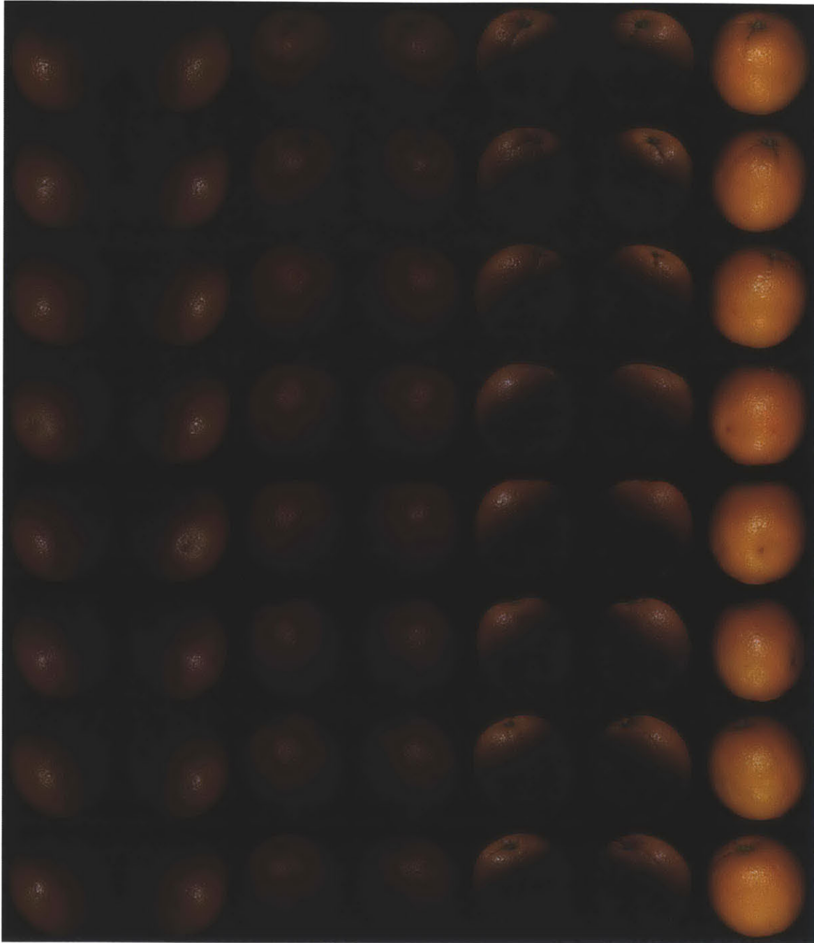
Figure 8-2: Texture images of an orange, covering all six lighting angles and all eight turntable angles.
