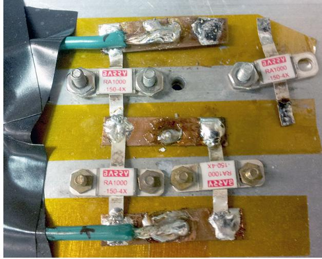
Figure 3-3: Picture of load resistor corresponding to 75% power
