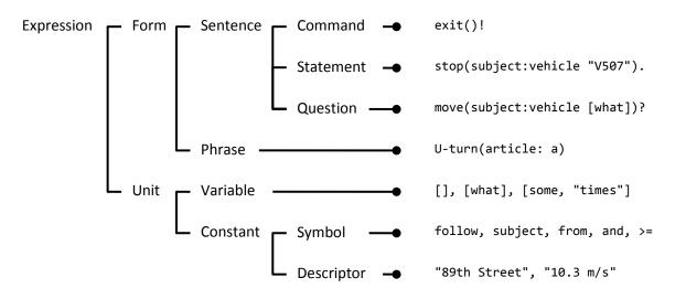
Forms have an optional Function (exit, stop, move and U-turn in the above examples) and zero or more Arguments, each of which has an optional Label (subject:vehicle and article: in the above examples) and a mandatory Value ("V507", [what] and a in the above examples). Labels have either or both a Syntactic Relation (subject and article in the above examples) and a Semantic Category (vehicle in the above examples); several Arguments in a
