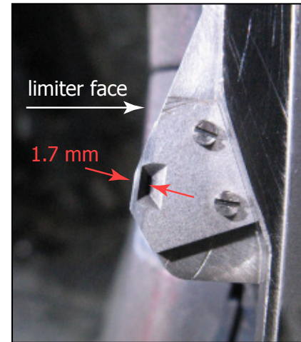
Figure 38: Retarding field analyzer mounted on the side of a limiter. Components are identical to that of the scanning retarding field analyzer, except that it is one-sided.
