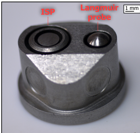
Figure 41: Front view of the ion sensitive probe sub-assembly.
