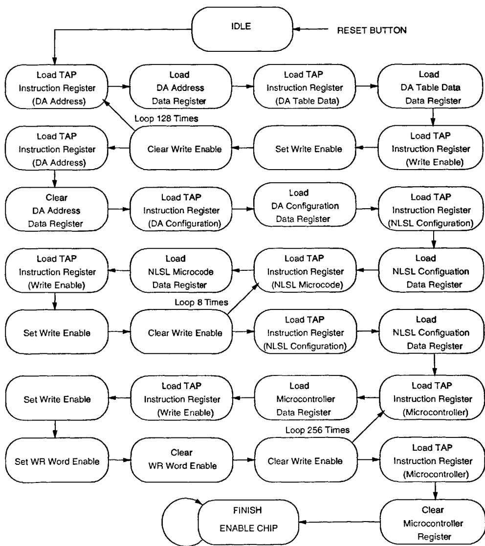
Figure 3-4: Programming Controller FSM State Diagram
