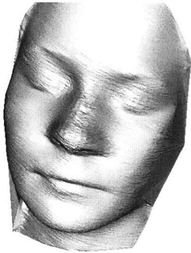
Figure 6-4: Shaded surface image of polygon mesh created from reconstructed surface of subject scanned
