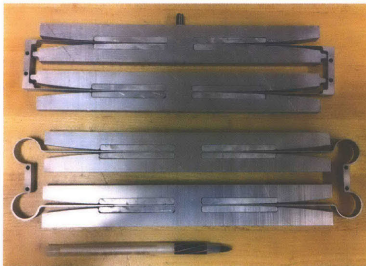
Figure 7-19: Fabricated aluminum load cells. Top: load cell without rotational springs. Bottom: Load cell with rotational spring.
