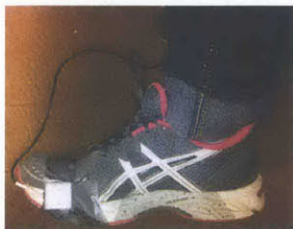
Figure 4-1: Experimental Set-up for collecting foot acceleration data
