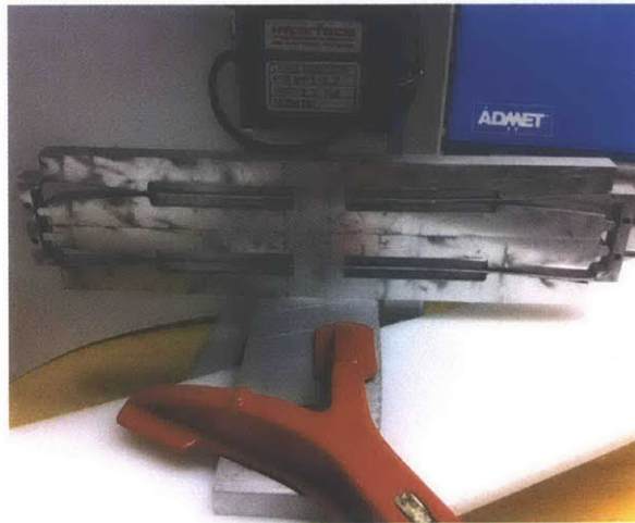
a) Load Cell with rigid connections, maximum compression
