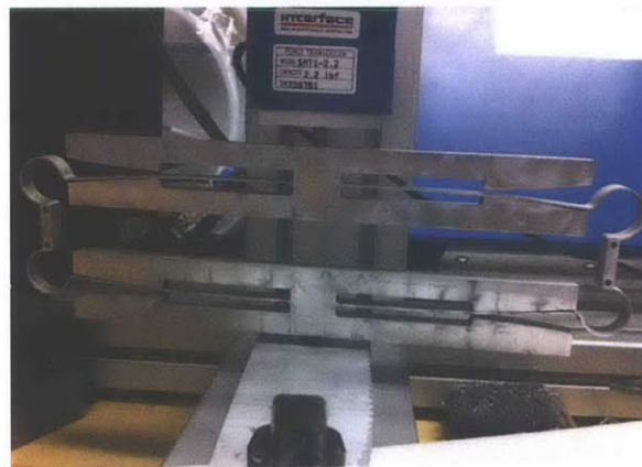
b) Load Cell with curved beam connections, maximum tension
