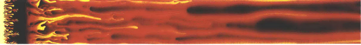
Figure 4-1: Snapshot of the concentration field during the alternating injection of more viscous (dark) and less viscous (light) fluids. Viscous fingering at the displacement front promotes mixing of the two fluids. At high viscosity contrast, however, a few dominating fingers coalesce to form persistent channels. These channels serve as preferential pathways for subsequent slugs of the less viscous fluid, inhibit transverse mixing, and shield growth of adjacent fingers. The displacement corresponds to a viscosity ratio M \approx 33 ( R = 3.5 ) and Péclet number Pe = 2000 . See supplementary videos [1].
