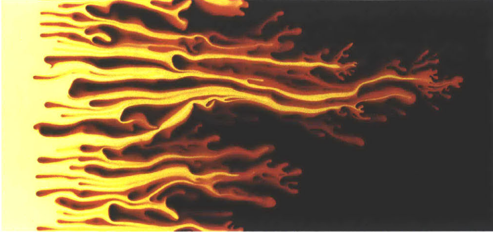
Figure 2-1: Snapshot of the concentration field during the unstable displacement of a more viscous fluid (dark) by a fully-miscible, less viscous fluid (light). The formation, splitting, and nonlinear interaction of viscous fingers induce disorder in the velocity field that affects the mixing rate between the fluids. The displacement corresponds to a viscosity ratio M = \exp(3.5) \approx 33 and Péclet number Pe = 10^4 . See also Video 1 in [1].
