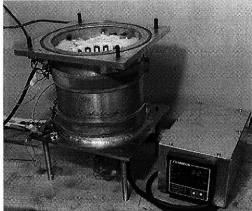
Figure 2.2: Picture of the small scale furnace developed at MIT.
