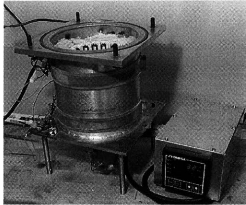
Figure 1.3: Small scale furnace built at MIT.
