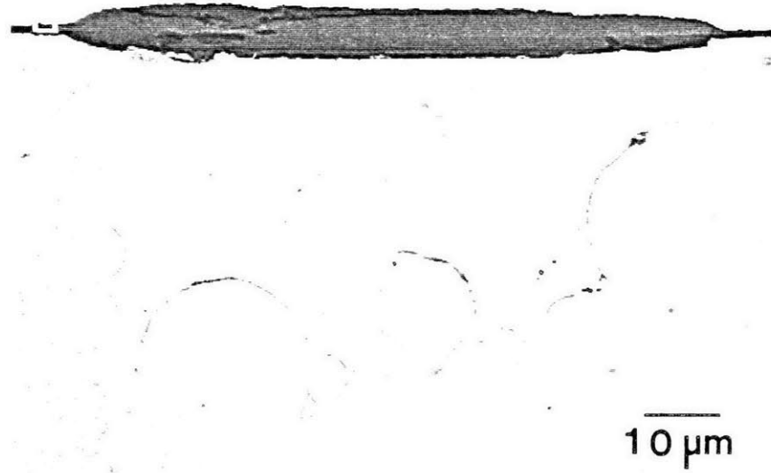
Figure 5.96—EPMA backscattered electron image of a cross-section through scale shown in figure 5.95.
