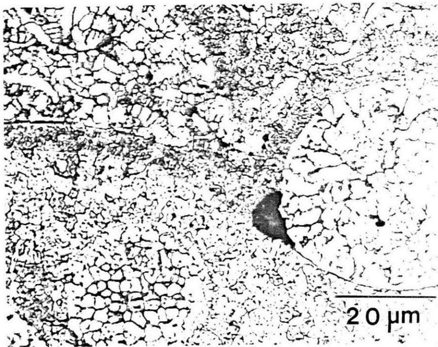
Figure 5.19—Optical micrograph of spray formed Fe-2.5Cr-2.5Al-1Ti-0.6B alloy processed at a 0.63m (25in) substrate position showing entrapped powder particles and splat boundaries.
