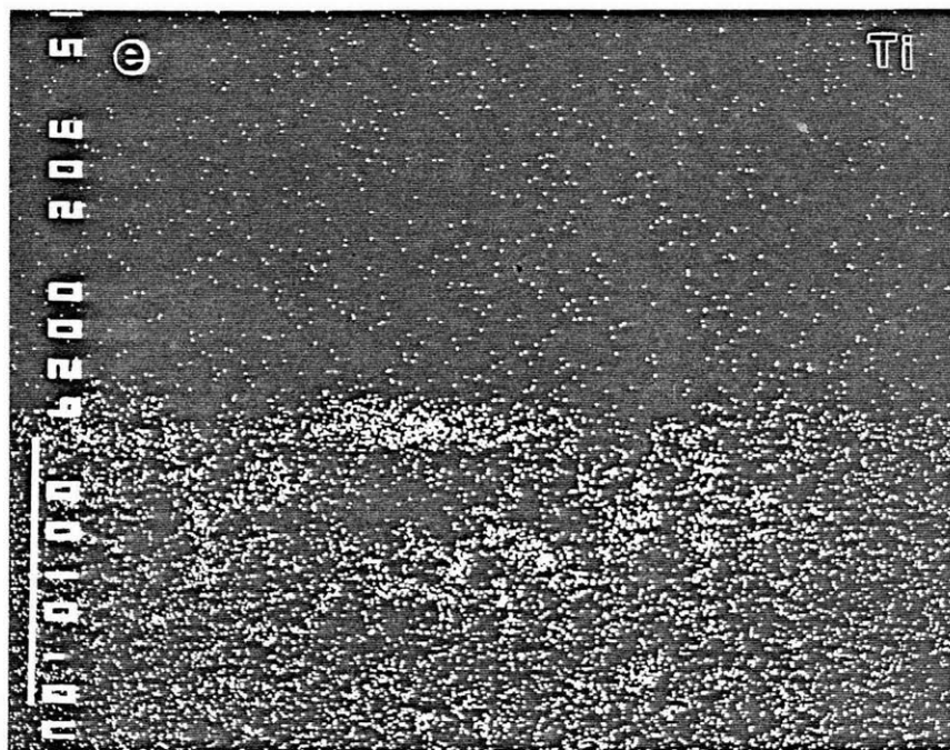
Figure 5.94 Cont.—(e) Elemental X-ray intensity map for titanium.
