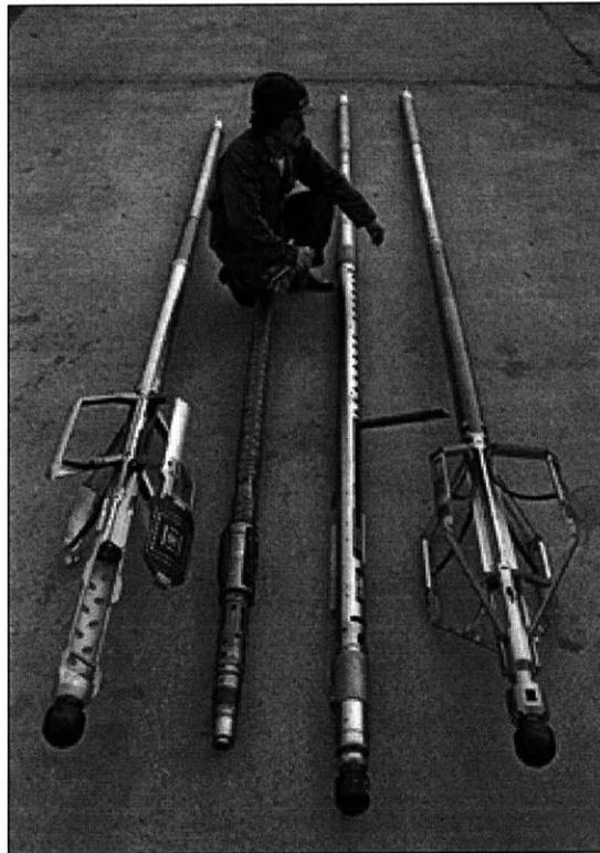
Figure 1.2: Schlumberger Logging Tools.<sup>1</sup>
