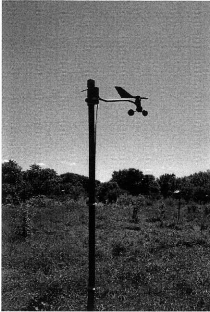
Figure 109 Wind monitoring instruments. A wire runs from the instruments to a laptop in the attic of the building.
