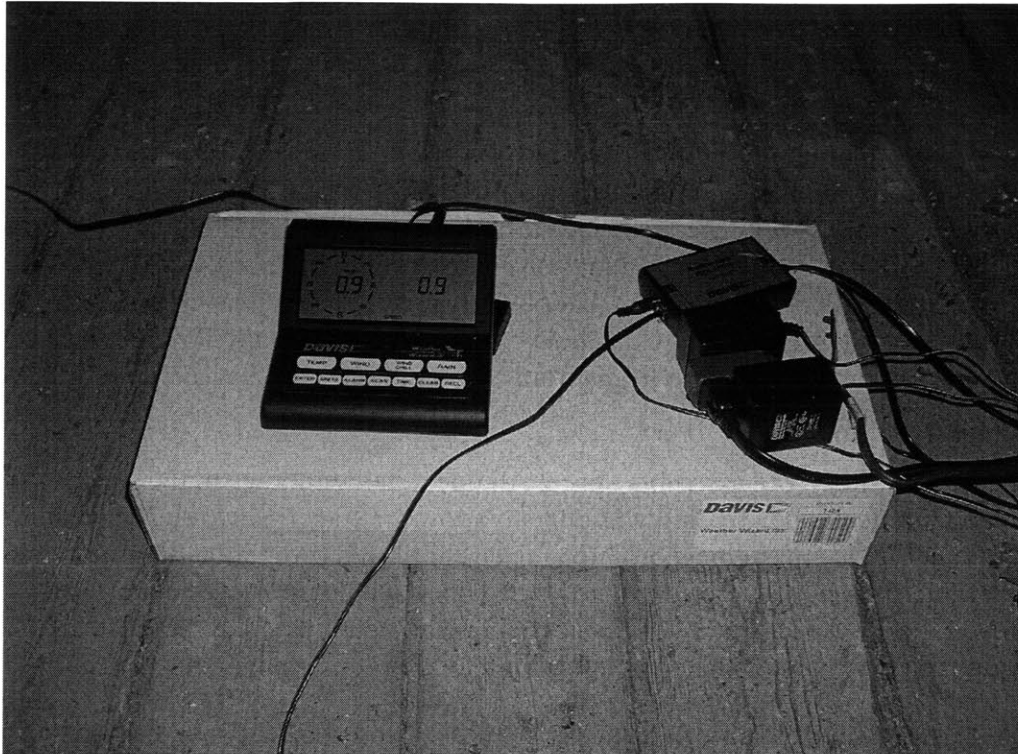
Figure 114 Weather station equipment. The device on the left is the weather station console. The device on the top right is a link isolator, which ensures a proper reference voltage for the wind station devices.
