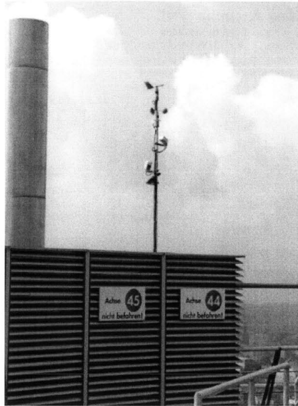
Figure 37 Roof-top weather station.
