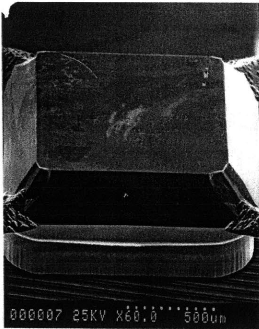
Figure 5.5 Front view SEM image of the convex coupling feature, (wafer 1). Traces of the convex corner compensating structures can be seen on the lower corners of the pyramid
