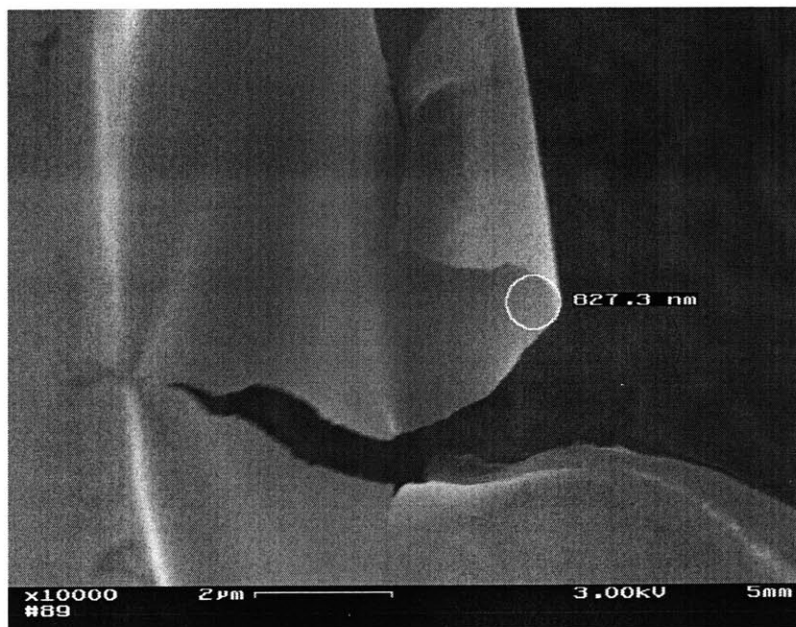
Figure 5-6: 50Å thick Cr curl with radius on the order of 400nm.
