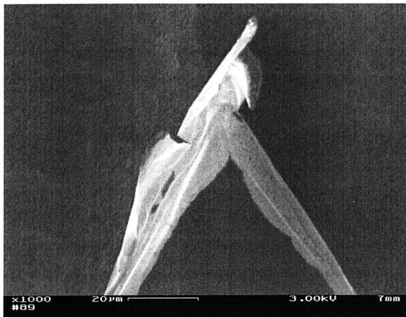
Figure 5-8: Close up of the tip of the triangle in Figure 5-7, showing curling only at the immediate edge.
