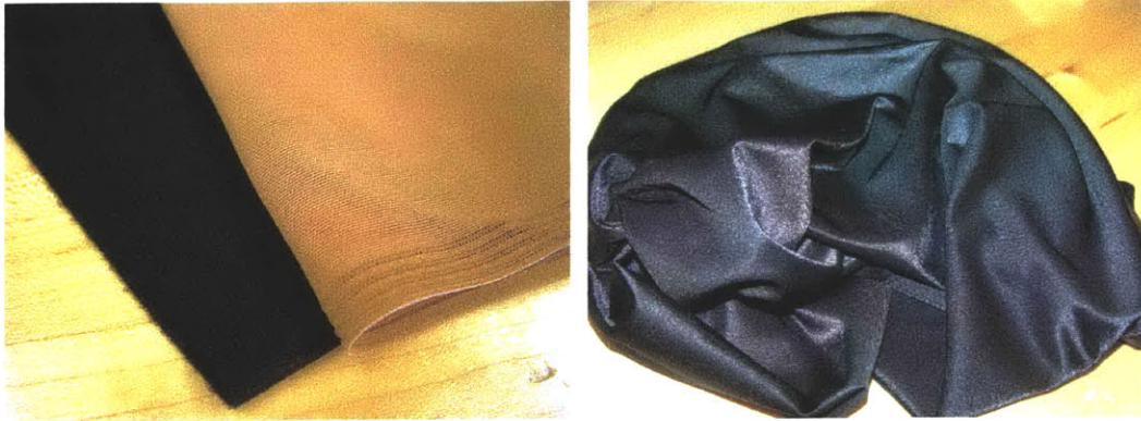
Figure 8-7. Two types of stretchable fabric. The black fabric is a spandex-like material, and the tan fabric is a nylon-like material (Powernet, Darlington Fabrics).
