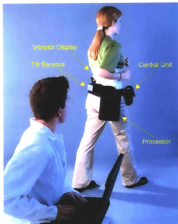
Figure 3-23. A balance prosthesis being developed by Wall and Weinberg (2003). Tactile feedback of body tilt in three dimensions is provided through a 3x16 array of vibratory tactors held against the torso (from Wall and Weinberg, 2003).
