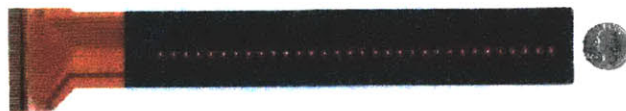
Figure 3-20. The Audiotact is an auditory prosthesis for the abdomen and contains 32 electrodes.
