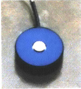
Figure 3-9. Tactile transducer (Model C1-97, Engineering Acoustics, Inc.).
