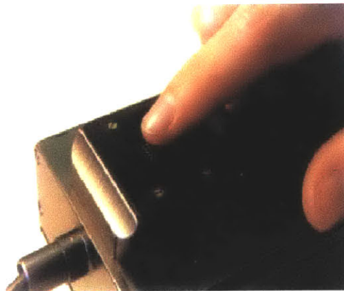
Figure 4-4. Dynamic display actuated by NiTi shape memory alloy wires; developed by TiNi Alloy, Co. (from Youngblut, 1996).
