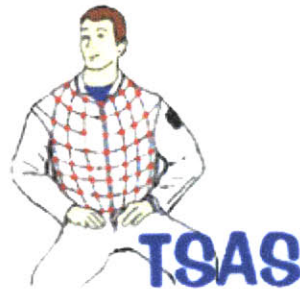
Figure 3-21. The Tactical Situation Awareness System (TSAS). Information on the orientation and movement of the aircraft is transmitted to the pilot via a matrix of vibrotactile stimulators on the pilot's torso and limbs (NAMRL, 2000).
