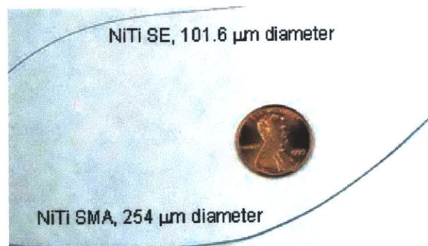
Figure 5-1. NiTi shape memory alloy and superelastic fibers used in experiments. The SMA fiber is 254 \mu\text{m} in diameter (Dynalloy, Inc., Flexinol™), has a 90°C transition temperature, and can generate a maximum of 180 MPa stress and 4% strain. The superelastic wire has diameter 101.6 \mu\text{m} .
