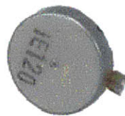
Figure 3-5. A pancake pager motor; an asymmetric weight attached to the motor inside the casing provides vibrational feedback.
