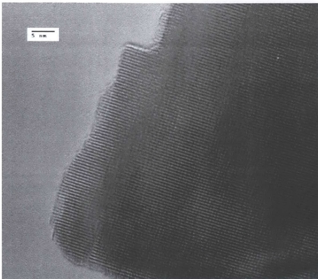
Figure 49. Typical TEM image of \text{Ca}_x\text{Mo}_6\text{Se}_8 particle. Crystalline planes are visible throughout the sample, all the way to the edge of the particle, as well as across the particle interior.
