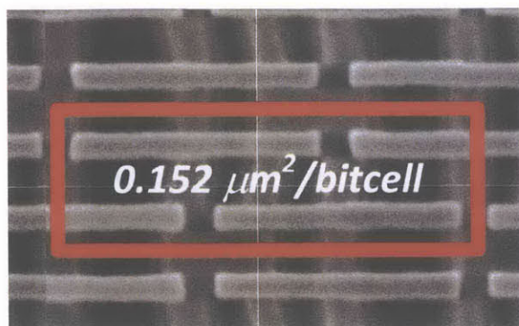
Figure 4-18: SEM picture of the 0.152\mu^2 6T bit-cell. This bit-cell is used in the 0.5Mb SRAM test-chip [7]. Courtesy of STMicroelectronics
