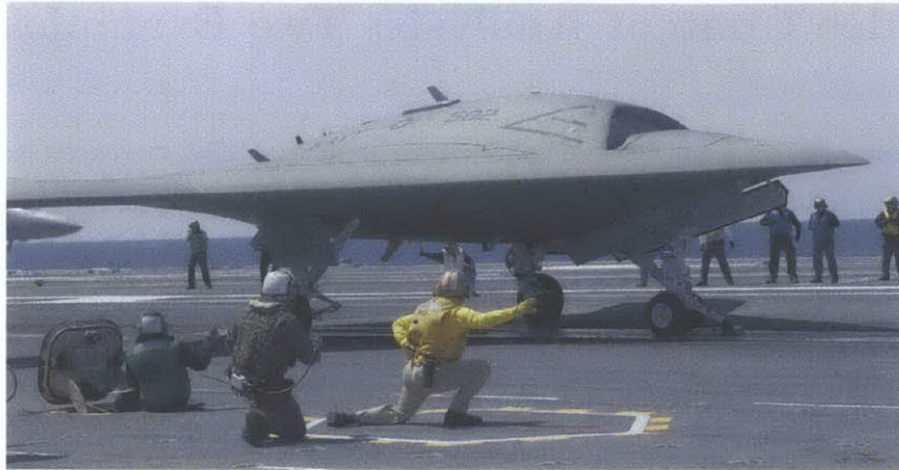
Figure 1-1: The US Navy plans to deploy drones to aircraft carriers by 2019. Shown above is the Northrop Grumman X-47B designed for carrier-based operations. Our ultimate goal is to enable drones to understand the same visual vocabulary of aircraft handling signals currently used for communication between pilots and aircraft marshallers.
