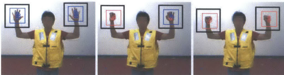
Figure 2-7: Search regions around estimated wrist positions (black rectangles) and clustering of multiple classification results. Our search region was 56 x 56 pixels (outer rectangles); the sliding window was 32 x 32 pixels (inner rectangles). Inner rectangles indicate clustered results (blue/red: palm open/close), and small circles are individual classification results (best viewed in color).
