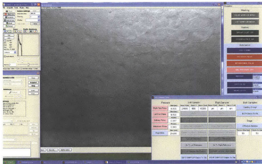
Figure 4.6: SCS control software differed significantly from the versions used for SCE (Chapter 3, Figure 3.6), partially because fewer parameters needed to be varied and partially because of different hardware (new camera). By this point in the automation development, less flexibility was needed to experiment with manual positioning of long-travel stages so options for these were removed as well.
