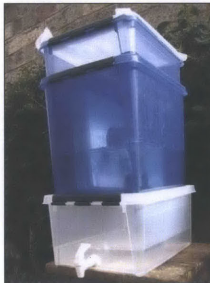
Figure 3-2: Gravity Driven Membrane (Source: Peter-Varbanets, et al., 2010)
