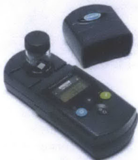
Figure 4-16: Hach Pocket Colorimeter II
