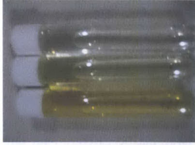
FIGURE 1 - COLILERT (NEGATIVE AND POSITIVE TOTAL COLIFORM) FIGURE 2 (COLILERT (NEGATIVE AND POSITIVE E. COLI )
