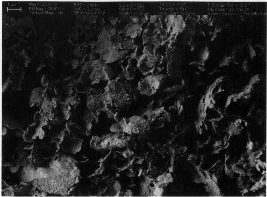
Figure 5.33 Cryo SEM image of Leached GOM EI hydrated with distilled water in a slurry state
