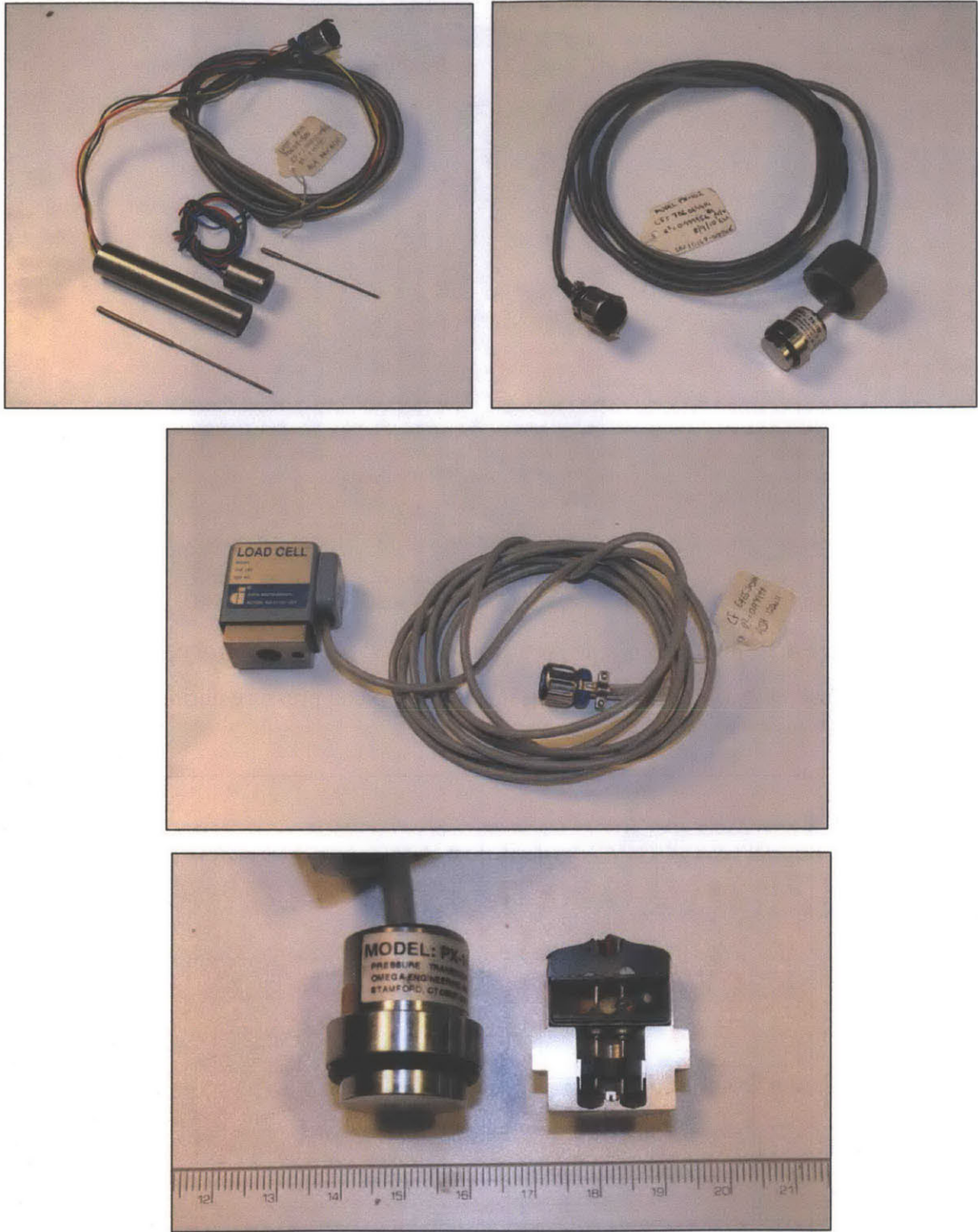
Figure 4.1 Electronic Transducers used during the testing program. Top Left: Trans-Tek LVDT's, Top Right: 0 – 200 psi capacity Pressure Transducer, Middle: 500 lb Load Cell, Bottom: Close-up of pressure transducer and section through one showing internal components (Horan, 2012)
