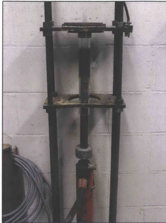
Figure 3.38 Hydraulic cylinder used to extrude a resedimented specimen from the consolidometer. This device is used when the resedimentation stress exceeds 0.5MPa
