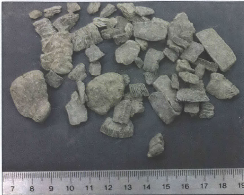
Figure 3.9 Size and color of GOM Upper Interval drill cuttings after removal of drilling fluid
