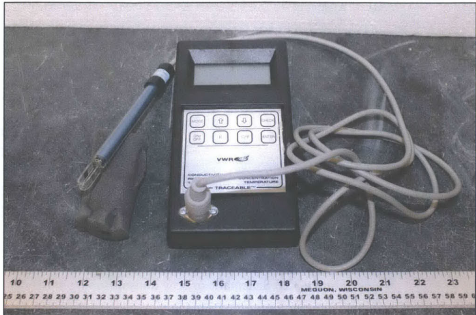
Figure 3.22 Conductivity Meter and associated probe used to measure the salinity of the bath water
