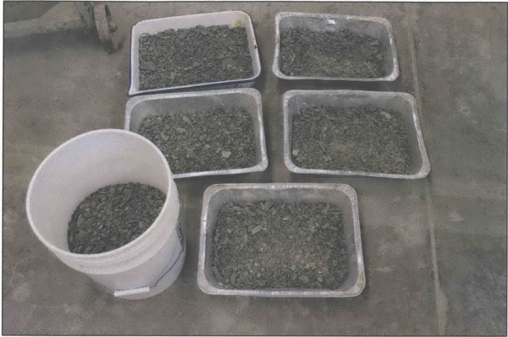
Figure 3.27 Cleaned GOM Upper placed in trays for oven drying to reduce moisture content to a level suitable for grinding in the GPX Disk Grinder
