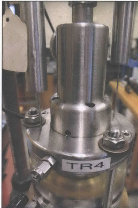
Figure 4.8 Trautwein CRS cell showing overflow hole which allows any water passing the piston seal to exit the device prior to contacting the roller bearings positioned higher in the piston column
