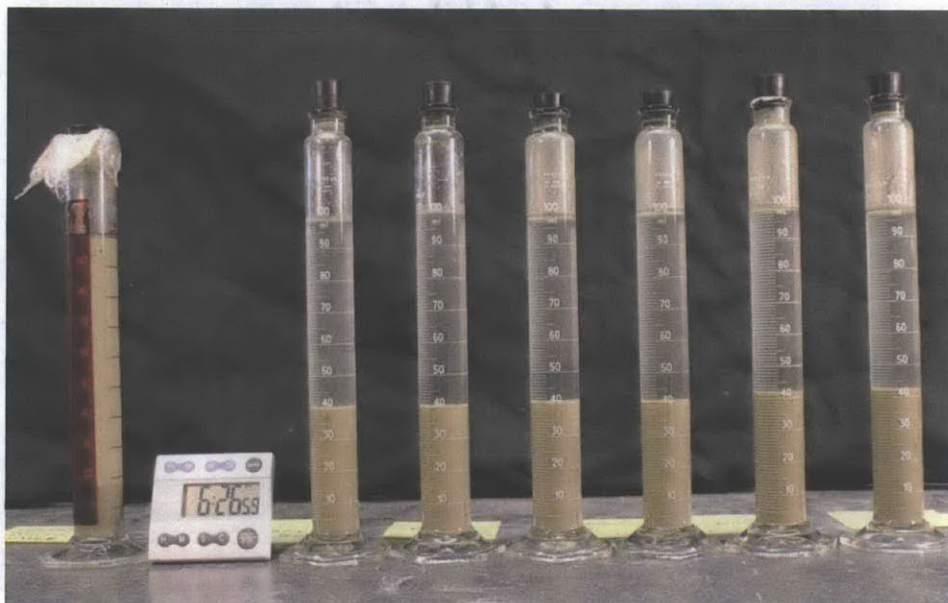
Figure 5.2 Sedimentation test performed on leached BBC powder. Salinities from L-R: 0 (distilled water) 1, 4, 16, 64, 128 & 256 g/l NaCl. 5 grams of soil used in each tube (Horan, 2012)
