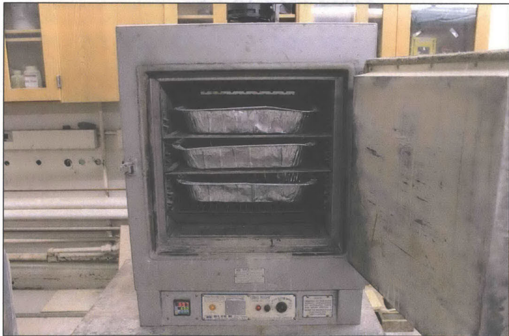
Figure 3.28 Trays of soil chunks placed in oven set at a temperature of 60° Celsius
