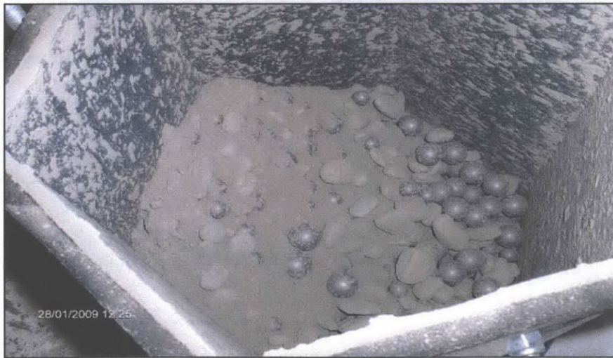
Figure 3.15 Ball Mill Grinder, Top: Rotating hexagonal steel drum powered by electric motor, Bottom: View inside drum of soil and steel ball mixture (Jones, 2010)
