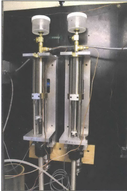
Figure 4.2 Pressure Volume Actuators (PVA's) used to control cell (left) and pore (right) pressures during triaxial testing in addition to cell pressure during CRS testing.
