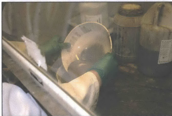
Figure 3.25 Removal of drilling fluid from GOM Lower. Top: First addition of Toluene to soil chunks, Middle: Sieving off toluene/drilling fluid mixture using #20 sieve, Bottom: adding toluene mixture back to soil chunks for secondary cleaning with drilling fluid at base of bowl removed
