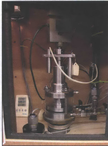
Figure 4.11 CRS Cell TR4 under test conditions. Temperature is maintained at a constant 25.3° C within the enclosure
