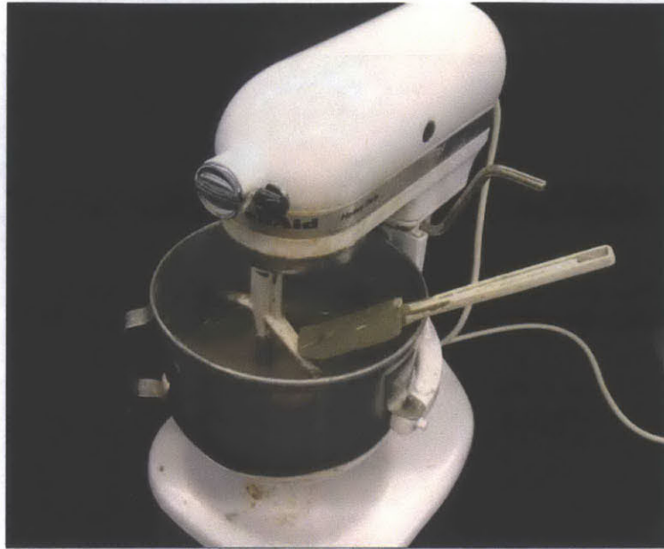
Figure 3.32 Kitchen aid mixer used to mechanically agitate soil/water mixture into a slurry
