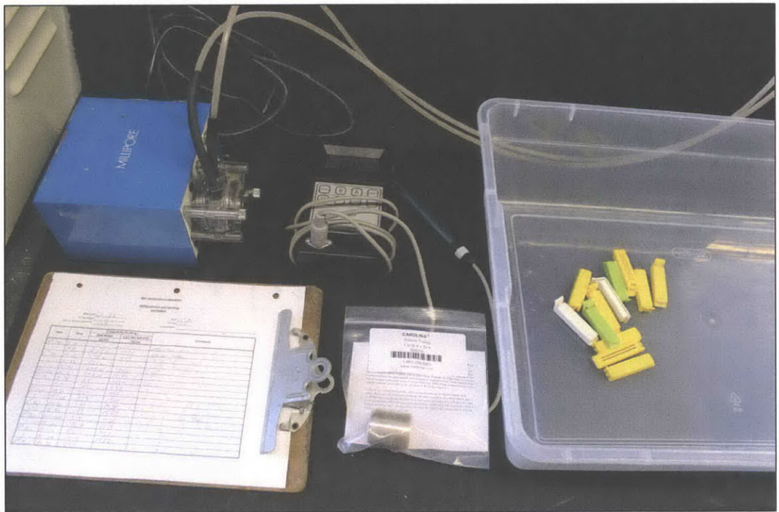
Figure 3.19 Equipment required for leaching the salts from soil using dialysis tubing
