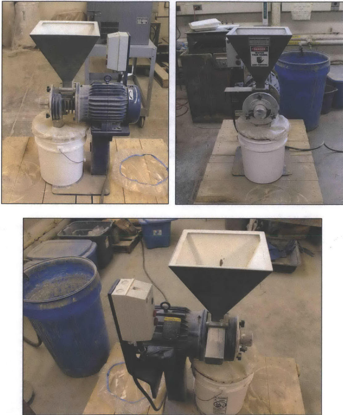
Figure 3.29 GPX Disc Grinder used in processing both GOM Upper and GOM Lower
