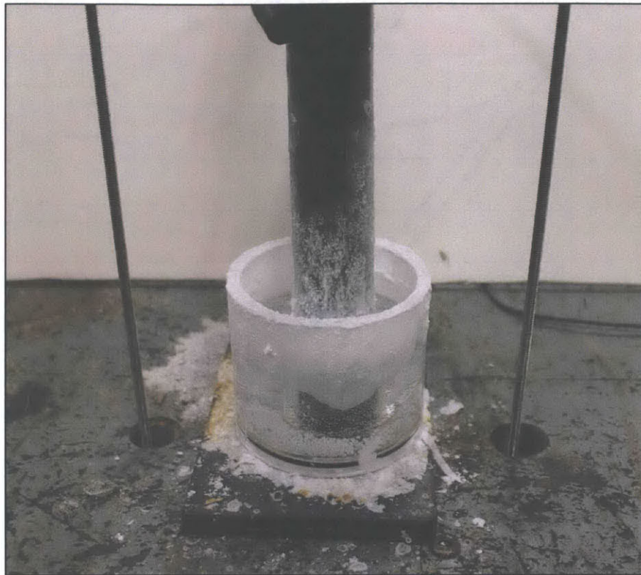
Figure 3.42 Issue of salt precipitating out of solution when resedimenting with high pore fluid salinities (soil shown is GOM EI resedimenting with a pore fluid salinity of 256g/L)
