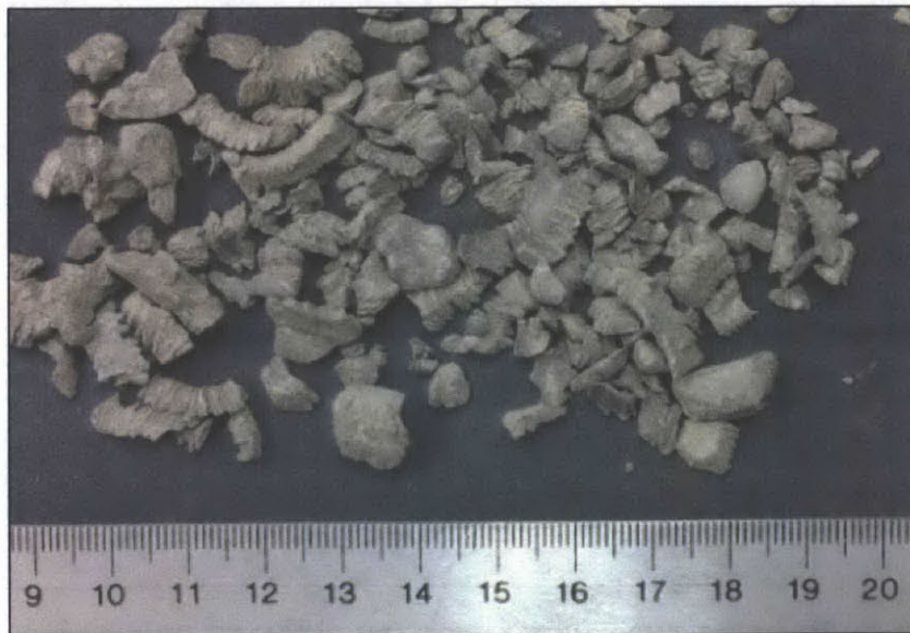
Figure 3.10 Size and color of GOM Lower Interval drill cuttings after removal of drilling fluid
