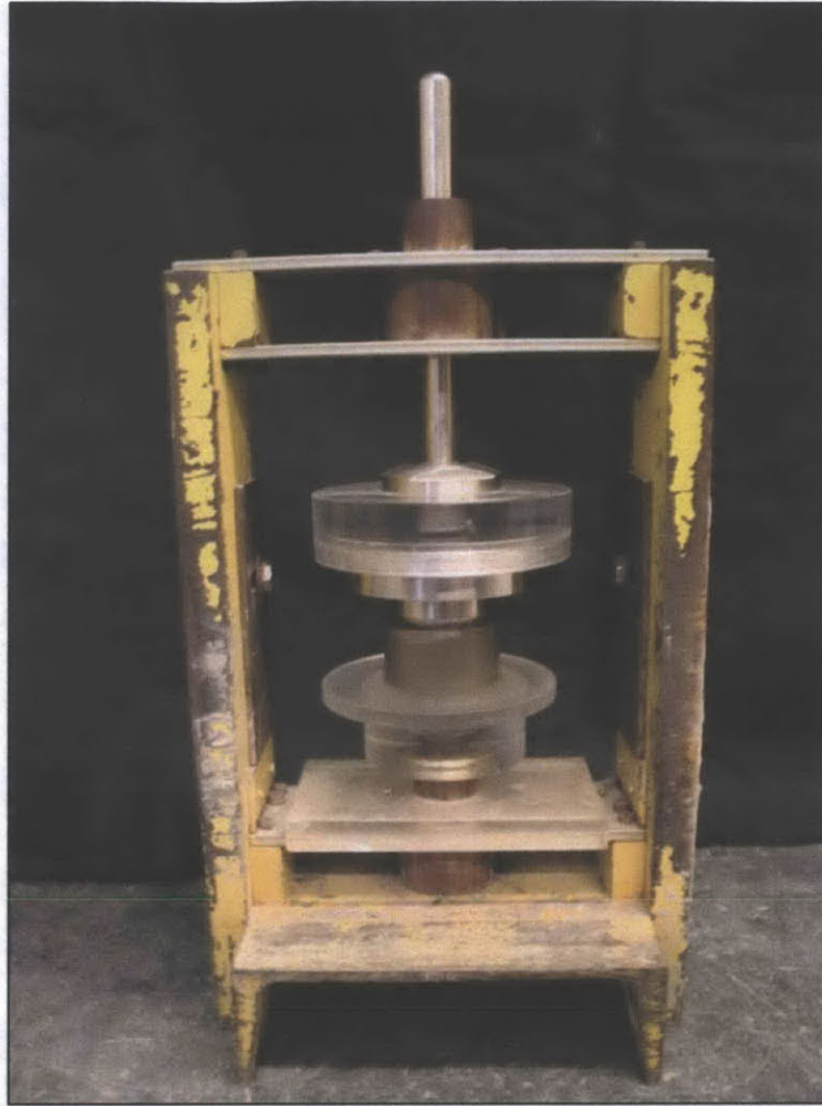
Figure 4.22 Trimming device with CRS trimming ring placed upside down concentrically on resedimented sample ensuring equal amount of soil for trimming around perimeter
