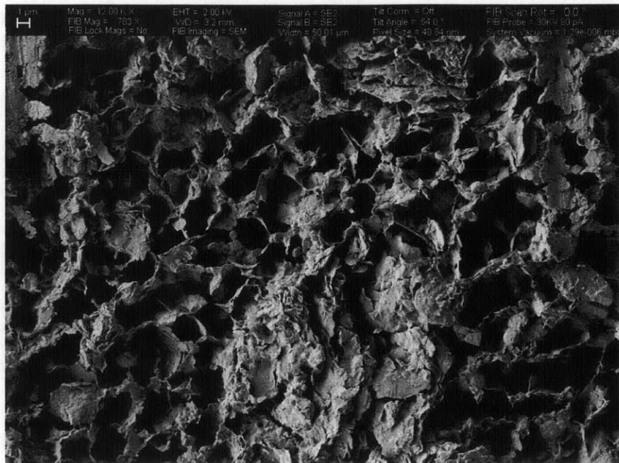
Figure 5.35 Cryo SEM image of GOM EI in a slurry state. Pore fluid salinity is 64 g/L
