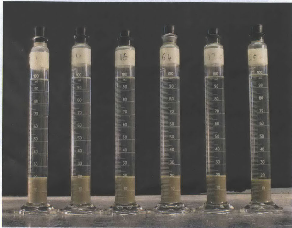
Figure 5.1 Sedimentation test performed on natural BBC Series IV powder. Salinities from LR: 1, 4, 16, 64, 128 & 256 g/l NaCl. 5 grams of soil used in each tube (Horan, 2012)
