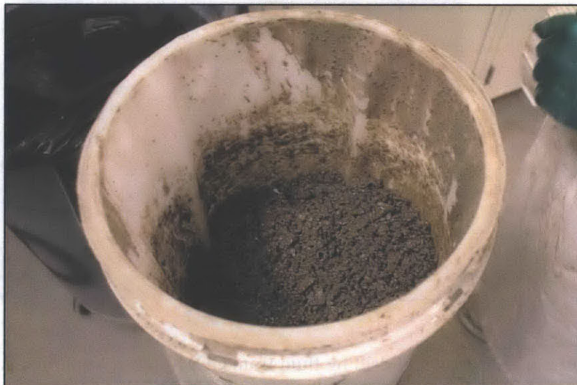
Figure 3.24 Condition of GOM Lower with each chunk of soil coated in drilling fluid prior to cleaning
