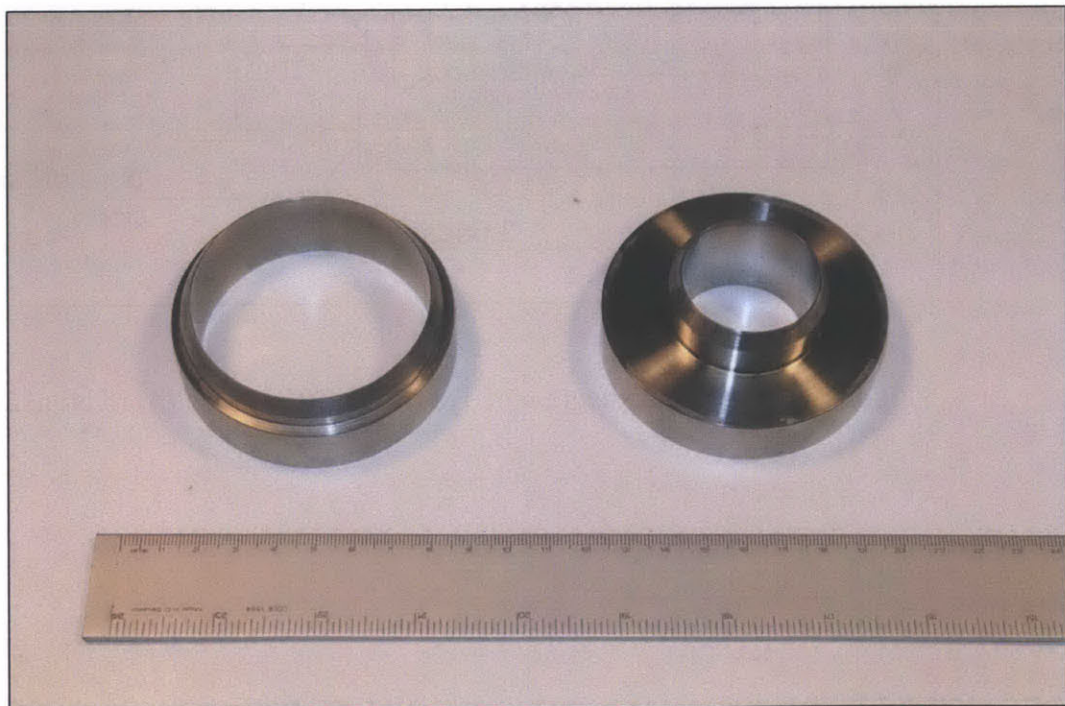
Figure 4.5 CRS trimming rings, Left: Standard Trimming Ring, Right: Trimming ring used in this research (Horan, 2012)
