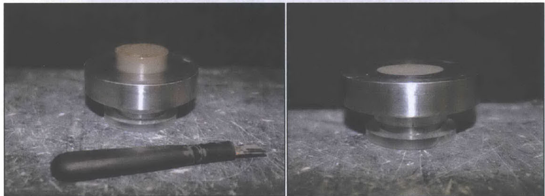
Figure 4.23 Trimming GOM EI sample into small diameter CRS ring, Top: Removing excess along the ring taper, Bottom Left: Positioning soil with plastic recess tool, Bottom Right: Final trimming with razor blade to ensure a level surface
