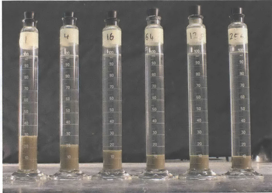
Figure 5.3 Sedimentation test performed on GOM EI powder. Salinities from L-R: 1, 4, 16, 64, 128, 256 g/l. 5g of soil in each tube
