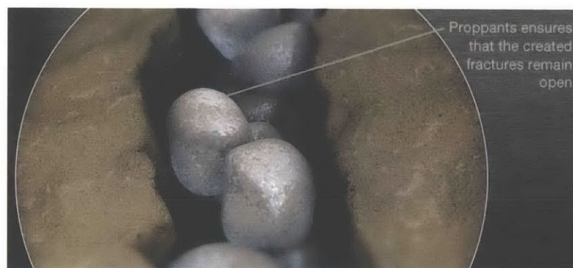
Figure 3: A zoomed-in view of a microfracture in rock that is held open by grains of sand or of a small, manufactured solid. This solid is known as a “proppant.” (Image source: http://www.wintershall.com/en/press-news/domestic-production.html )
