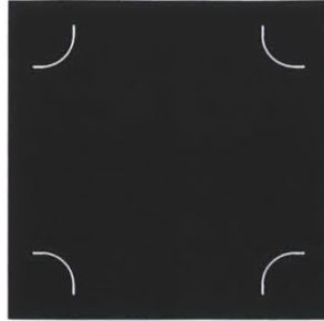
Figure 3-7: The insulating layer only has one mask to define the etch lines on both sides for the deep anisotropic etch in hydrofluoric acid.
