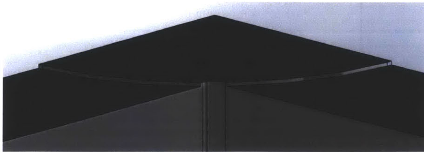
Figure 2-5: An isolated view of a frame base layer corner where a pedestal is defined to prevent bonding anywhere but at the corners.
