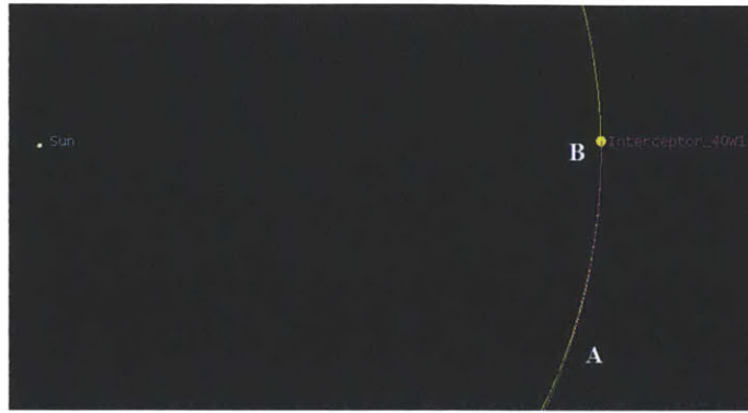
Figure 5-15: Last 20 days of maneuvering represented by purple arc; NEO orbit shown in yellow. HCI frame.
