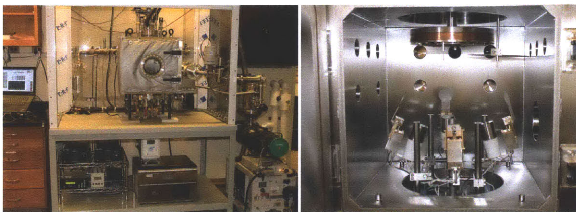
Figure 1-5. (Left) Full reactor setup. The valves and heaters are controlled through the computer control system on the left. Underneath the chamber are various controllers for the evaporation sources, butterfly valve, and turbopump. (Right) Inside of the new oCVD chamber. The inverted stage on the top is able to rotate. There are four evaporation sources on the bottom, each with its individual shutter (shown open).
