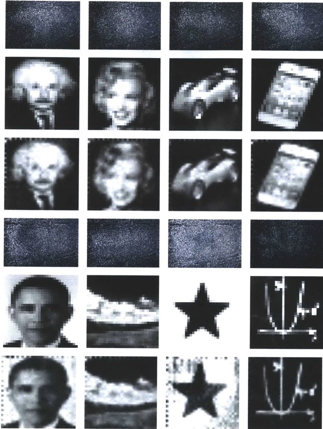
Figure 5-3: Sparkle vision through glitter board: Row 1 and 4 present the sensor output. Row 2 and 5 present the reconstruction, and Row 3 and 6 present the result of “sparkle vision”
