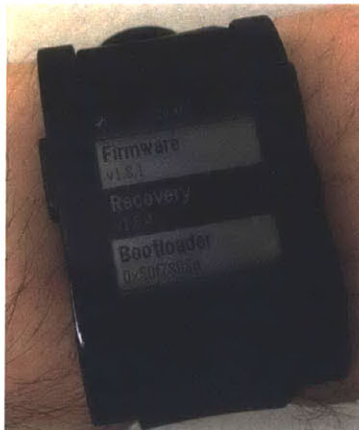
Figure 2-5: Watch used in our wearable system for user input (with the three buttons on the right) and output (via glanceable text display or vibration-encoded text).
