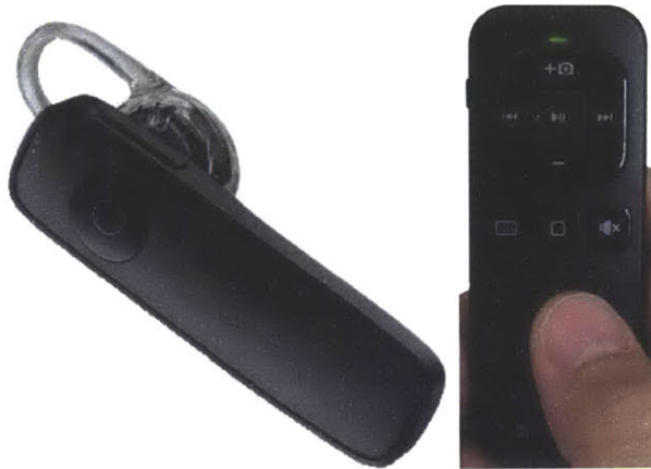
Figure 2-6: Optional accessories for our wearable system. Left: a Bluetooth headset for personal audio. Right: a Bluetooth remote placed within a pocket and used for discreet cueing. All buttons are mapped to a common function so that the wearer need only press against the outside of their pocket.
