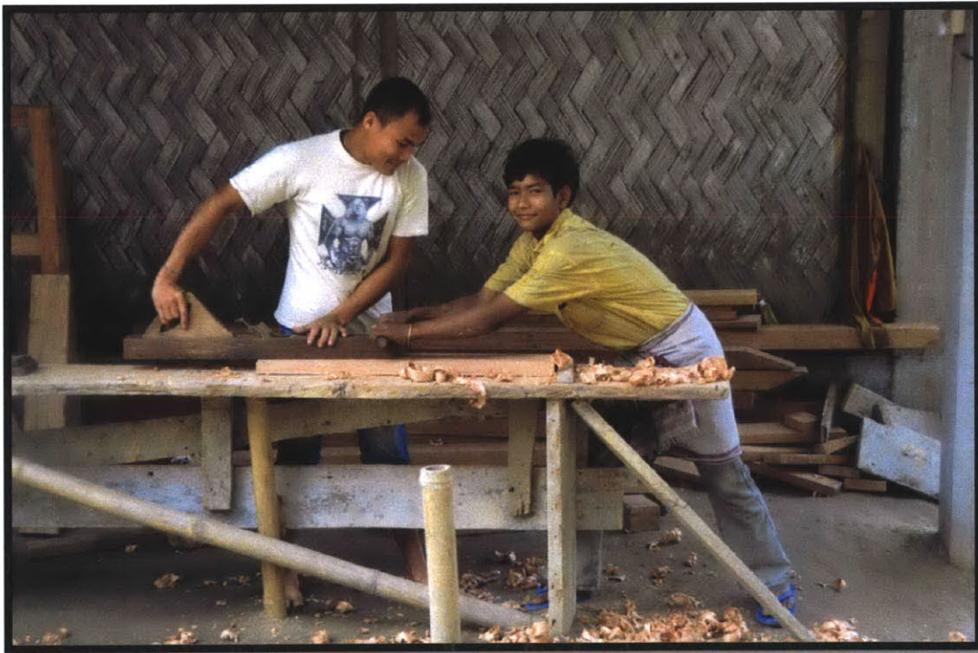
Figure 3.5: Carpenters using hand fabrication to work on wood piece
